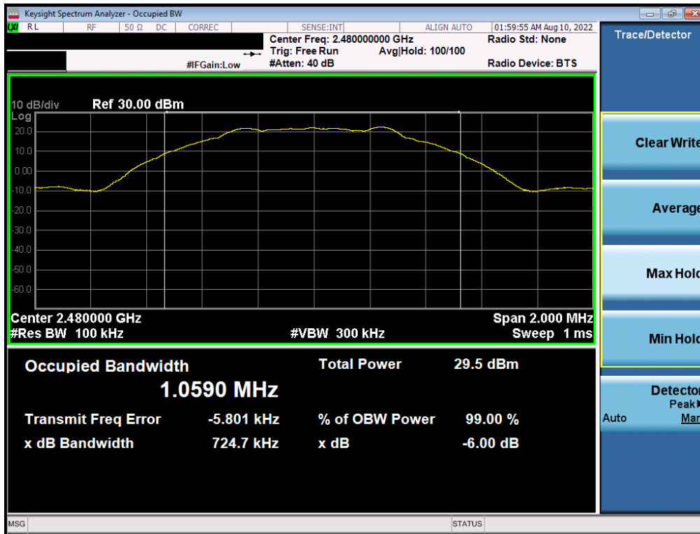
Plot 7-3. 6dB BW & 99% OBW Plot Antenna WF8 (Bluetooth (LE), 1Mbps, ePA – Ch. 39)
