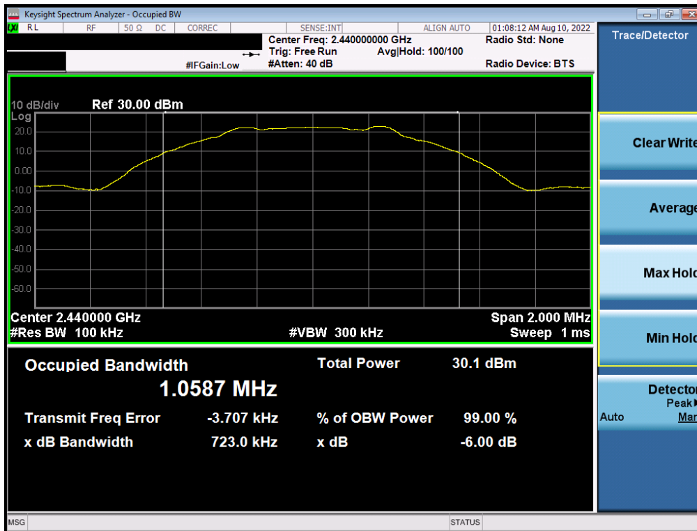
Plot 7-8. 6dB BW & 99% OBW Plot Antenna WF7 (Bluetooth (LE), 1Mbps, ePA – Ch. 19)
