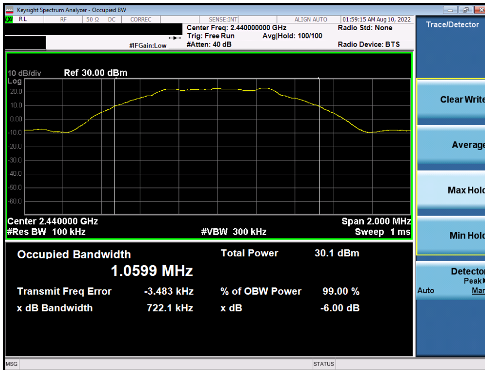
Plot 7-2. 6dB BW & 99% OBW Plot Antenna WF8 (Bluetooth (LE), 1Mbps, ePA – Ch. 19)
