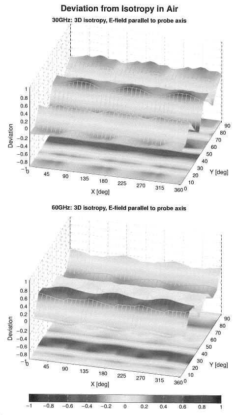
Probe isotropy for E<sub>tot</sub>: probe rotated  $\phi = 0^{\circ}$  to 360°, tilted from field propagation direction  $\vec{k}$ Parallel to the field propagation ( $\psi = 0^{\circ} - 90^{\circ}$ ) at 30 GHz: deviation within ±0.42 dB Parallel to the field propagation ( $\psi = 0^{\circ} - 90^{\circ}$ ) at 60 GHz: deviation within ±0.33 dB
