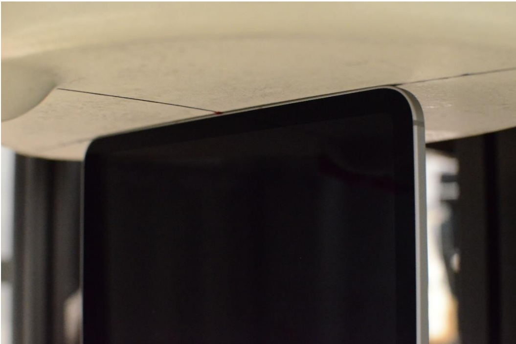
Body SAR Test Setup Photo 4: Bottom Edge at 0.0 cm
