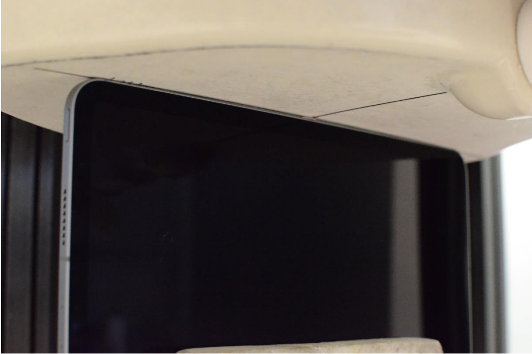
Body SAR Test Setup Photo 5: Right Edge at 0.0 cm
