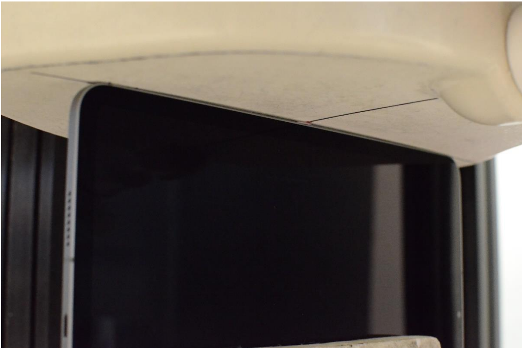
Body SAR Test Setup Photo 6: Left Edge at 0.0 cm
