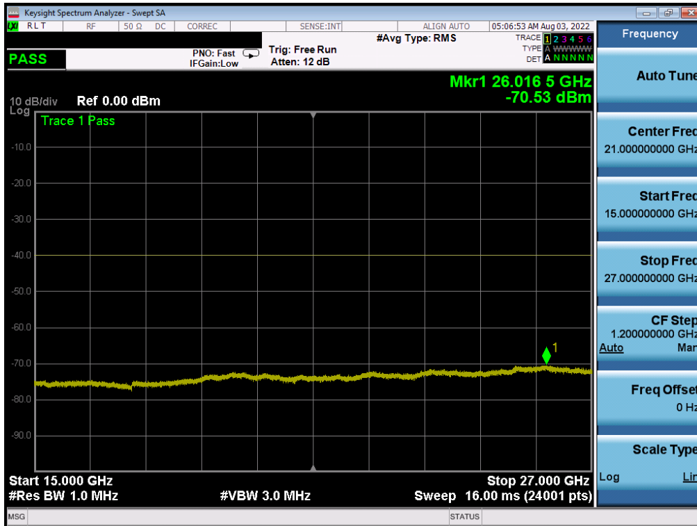
Plot 7-27. Conducted Spurious Plot (NR Band n48 - 40MHz QPSK - Mid Channel)
