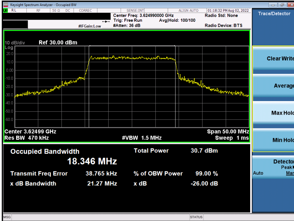
Plot 7-9. Occupied Bandwidth Plot (NR Band n48 - 20MHz 64-QAM - Full RB Configuration)
