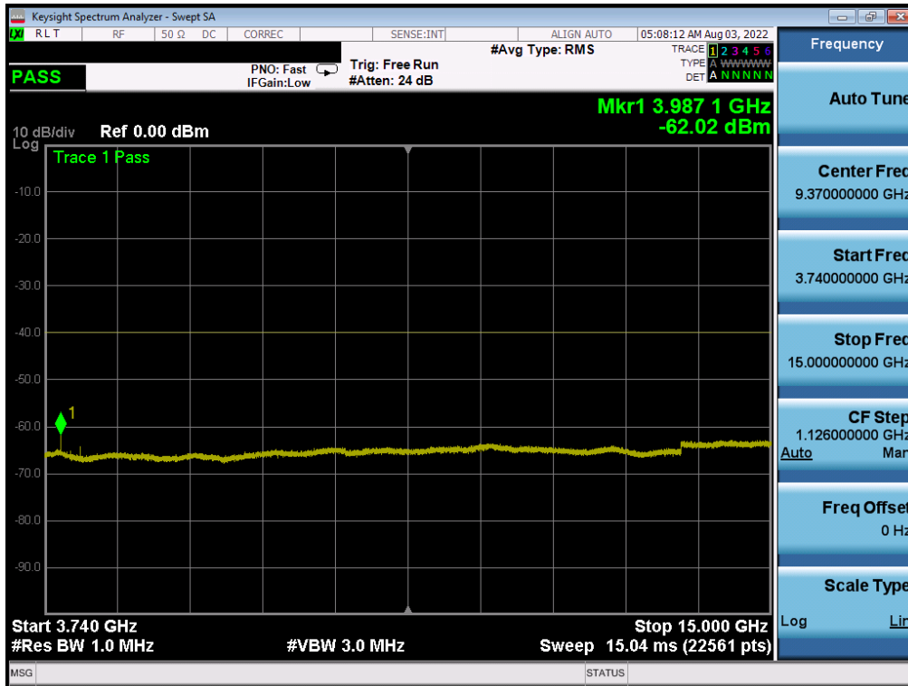
Plot 7-30. Conducted Spurious Plot (NR Band n48 - 40MHz QPSK - High Channel)
