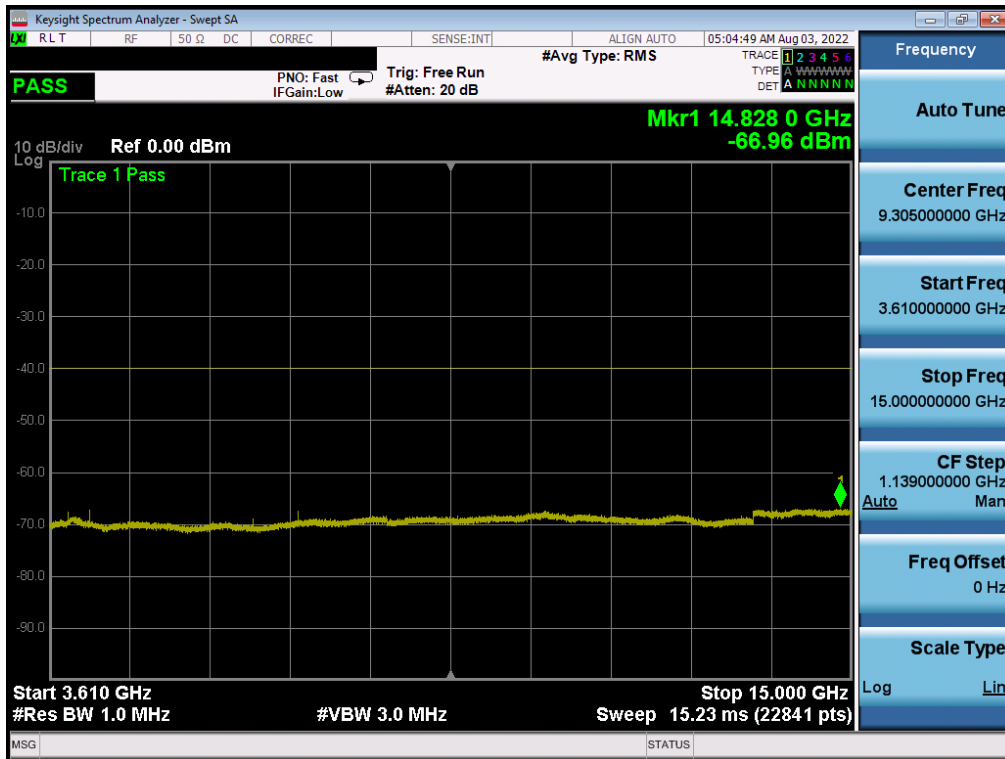
Plot 7-22. Conducted Spurious Plot (NR Band n48 - 40MHz QPSK - Low Channel)
