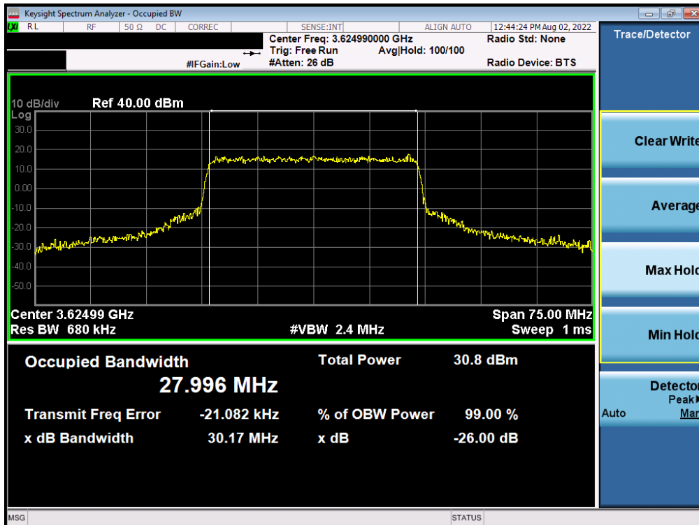
Plot 7-14. Occupied Bandwidth Plot (NR Band n48 - 30MHz 64-QAM - Full RB Configuration)
