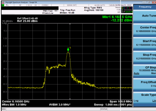
Plot 7-269. Power Spectral Density Plot SDM Antenna 5b (40MHz 802.11ax RU26 (UNII Band 5) – Ch. 43)
