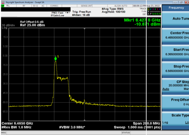
Plot 7-153. Power Spectral Density Plot Antenna 5b (80MHz 802.11ax RU26 (UNII Band 6) – Ch. 103)
