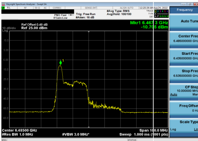
Plot 7-149. Power Spectral Density Plot Antenna 5b (40MHz 802.11ax RU26 (UNII Band 6) – Ch. 107)
