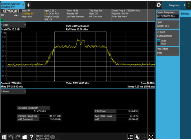
Plot 7-66. 26dB & 99% Bandwidth Plot Antenna 5b (20MHz 802.11ax RU26 (UNII Band 5) – Ch. 45)
