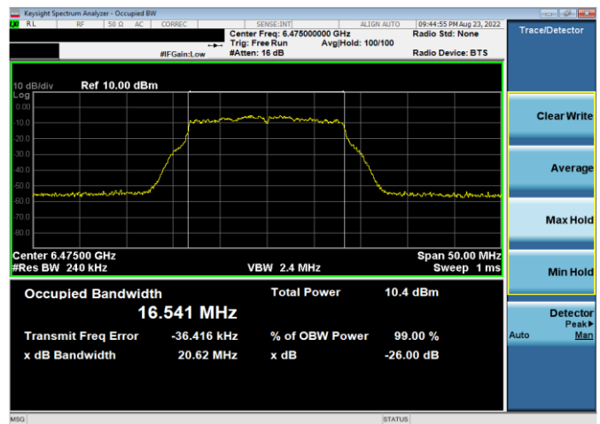
Plot 7-26. 26dB & 99% Bandwidth Plot Antenna 5b (20MHz 802.11a (UNII Band 6) – Ch. 105, 24Mbps)
