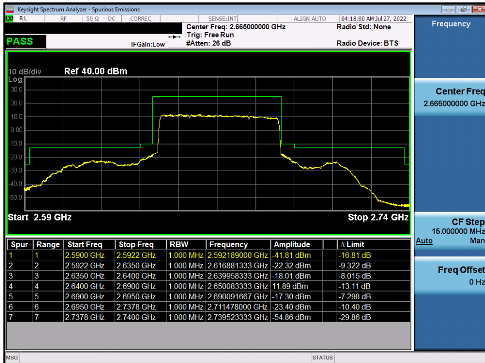
Plot 7-283. Upper ACP Plot (NR Band n41 - 50MHz DFT-s-OFDM \pi/2 BPSK - Full RB)
