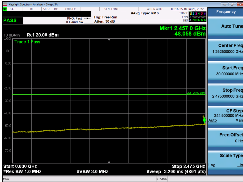
Plot 7-181. Conducted Spurious Plot (NR Band n7 - 40MHz DFT-s-OFDM QPSK - RB Size 1, RB Offset 0 - High Channel)
