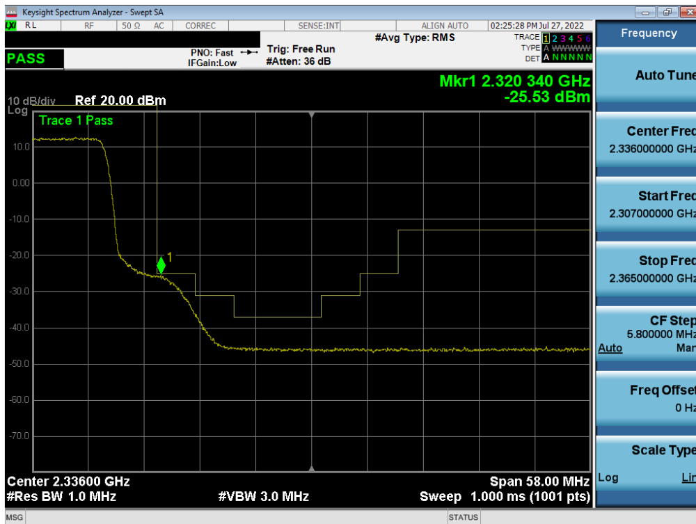
Plot 7-218. Extended Upper Band Edge Plot (LTE Band 30 - 10MHz QPSK – Full RB)
