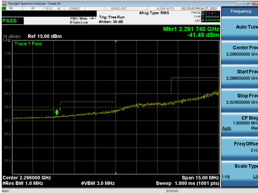
Plot 7-212. Extended Lower Band Edge Plot (LTE Band 30 - 5MHz QPSK – Full RB)
