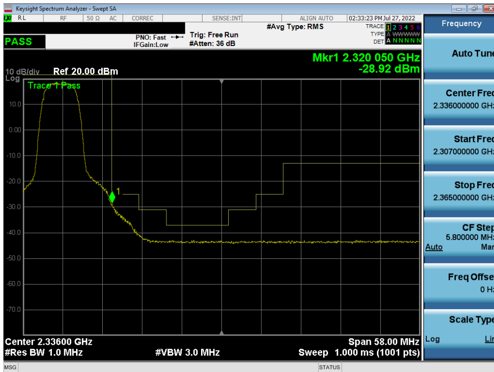
Plot 7-214. Extended Upper Band Edge Plot (LTE Band 30 - 5MHz QPSK – Full RB)
