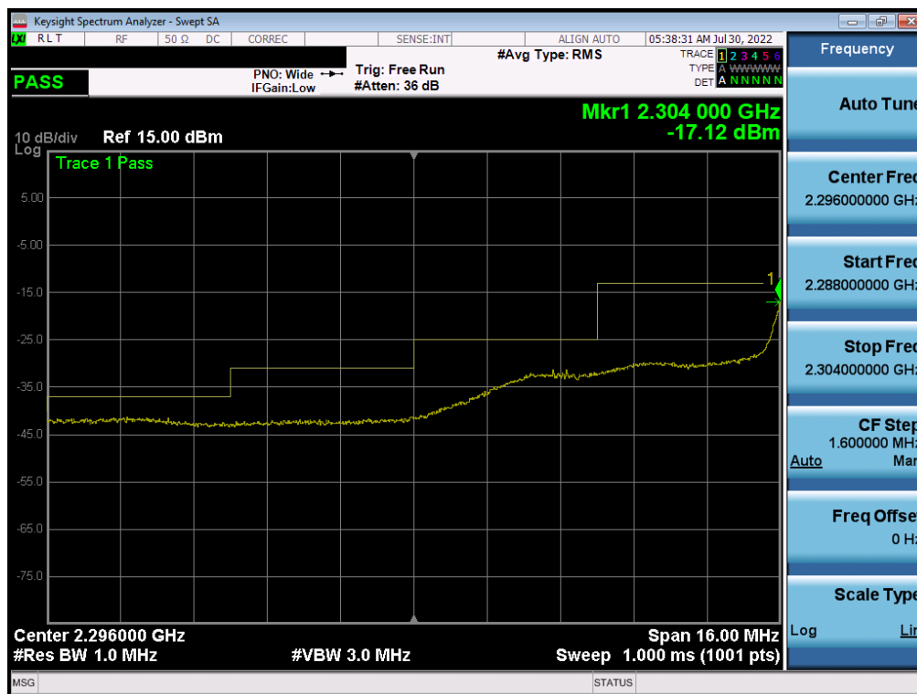
Plot 7-248. Extended Lower Band Edge Plot (NR Band n30 - 10MHz DFT-s-OFDM \pi/2 BPSK – Full RB)
