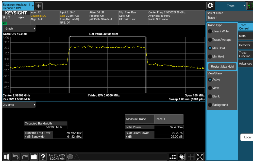
Plot 7-107. Occupied Bandwidth Plot (NR Band n41 - 60MHz DFT-s-OFDM QPSK - Full RB)
