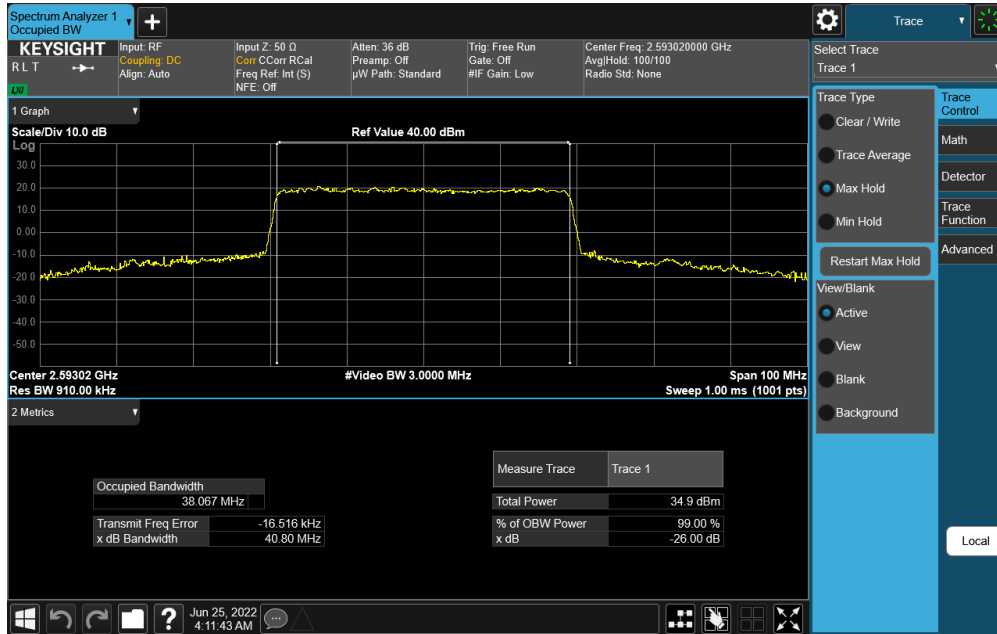
Plot 7-98. Occupied Bandwidth Plot (NR Band n41 - 40MHz CP-OFDM 16-QAM - Full RB)
