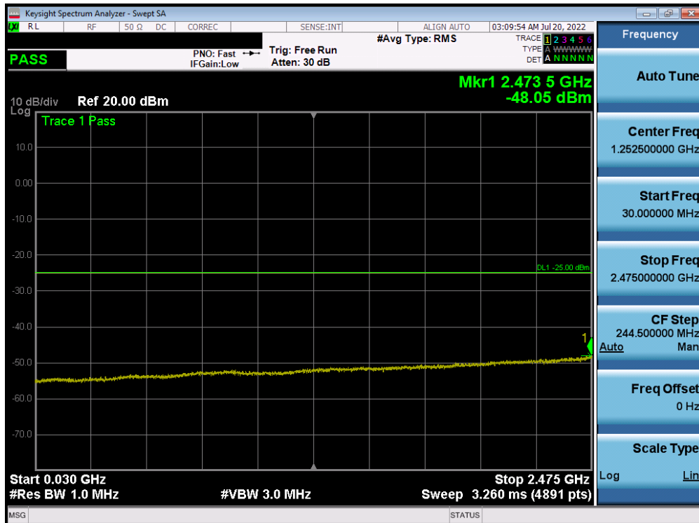
Plot 7-178. Conducted Spurious Plot (NR Band n7 - 40MHz DFT-s-OFDM QPSK - RB Size 1, RB Offset 0 - Mid Channel)
