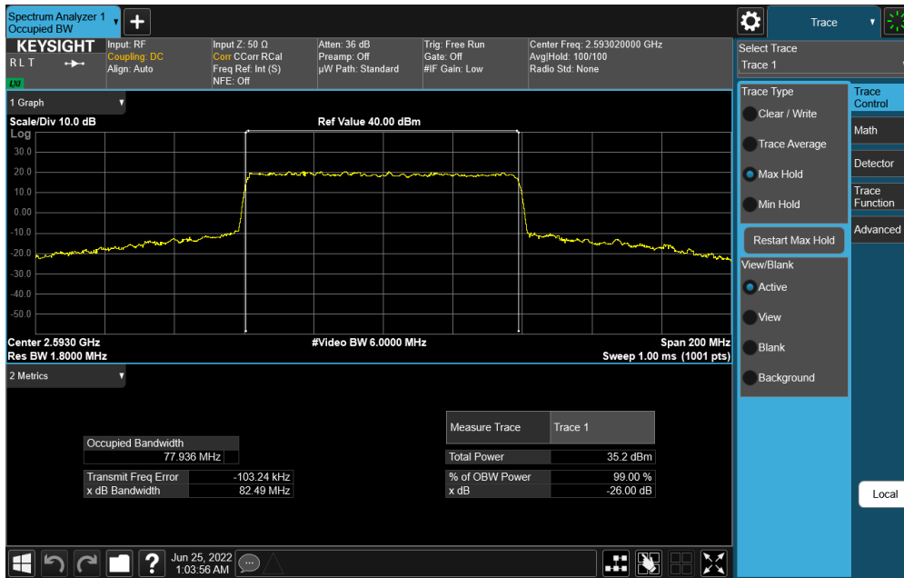
Plot 7-119. Occupied Bandwidth Plot (NR Band n41 - 80MHz CP-OFDM 64-QAM - Full RB)
