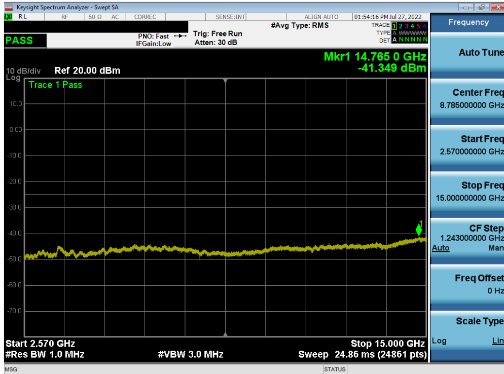
Plot 7-152. Conducted Spurious Plot (LTE Band 7 - 20MHz QPSK - RB Size 1, RB Offset 0 - Mid Channel)
