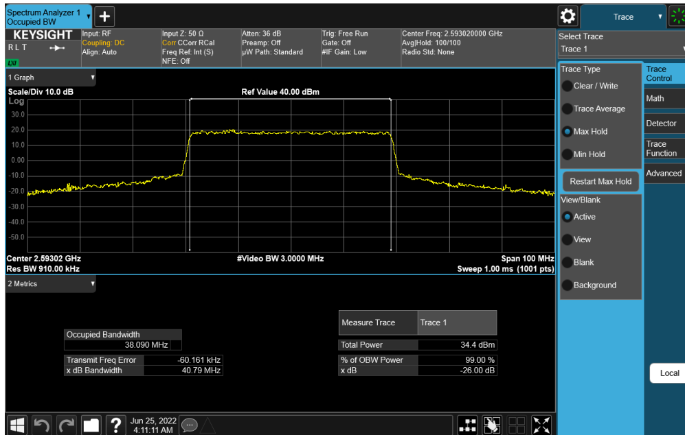
Plot 7-99. Occupied Bandwidth Plot (NR Band n41 - 40MHz CP-OFDM 64-QAM - Full RB)
