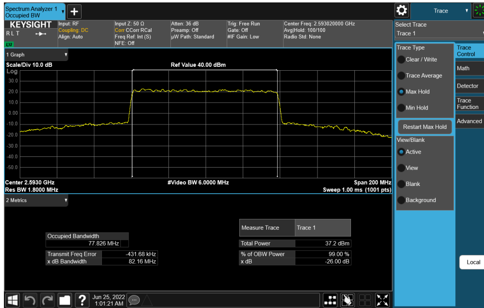
Plot 7-117. Occupied Bandwidth Plot (NR Band n41 - 80MHz CP-OFDM QPSK - Full RB)
