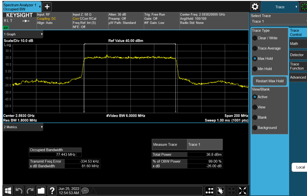
Plot 7-116. Occupied Bandwidth Plot (NR Band n41 - 80MHz DFT-s-OFDM \pi/2 BPSK - Full RB)
