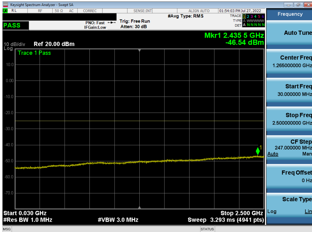
Plot 7-151. Conducted Spurious Plot (LTE Band 7 - 20MHz QPSK - RB Size 1, RB Offset 0 - Mid Channel)
