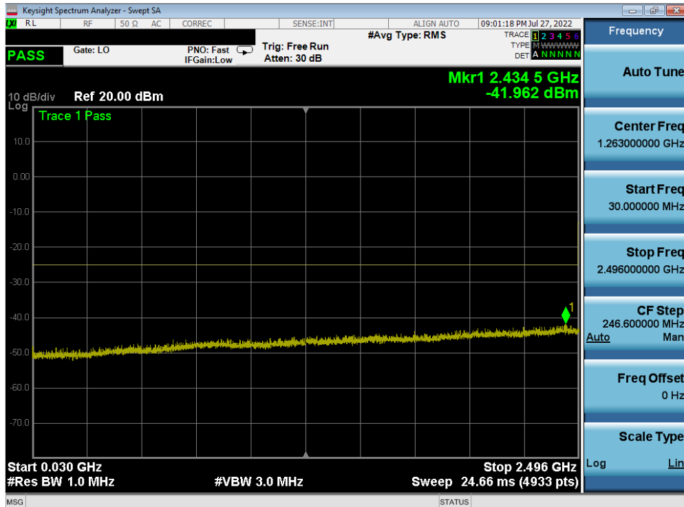
Plot 7-160. Conducted Spurious Plot (LTE Band 41 - 20MHz QPSK - RB Size 1, RB Offset 0 - Mid Channel)
