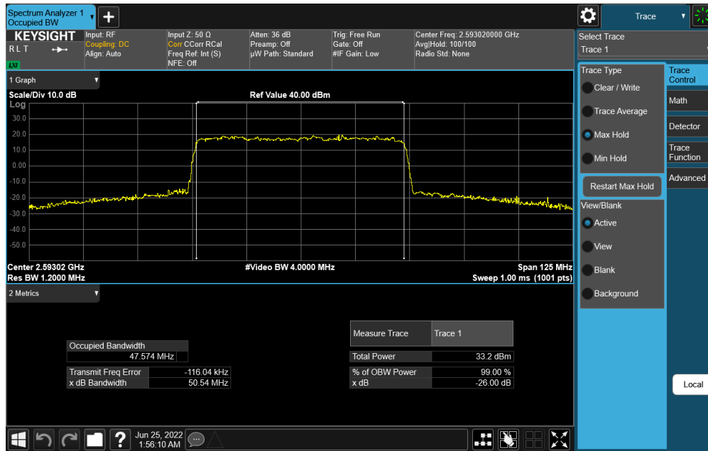
Plot 7-105. Occupied Bandwidth Plot (NR Band n41 - 50MHz CP-OFDM 256-QAM - Full RB)
