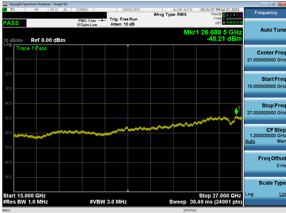
Plot 7-147. Conducted Spurious Plot (LTE Band 30 - 5MHz QPSK - RB Size 1, RB Offset 0 – High Channel)
