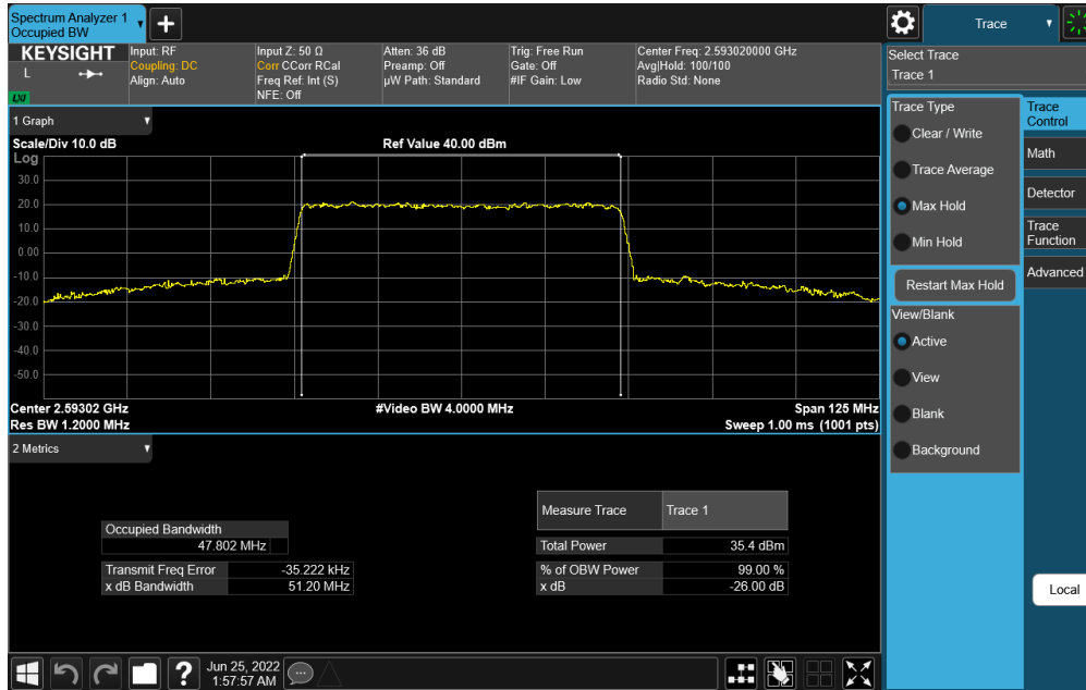
Plot 7-102. Occupied Bandwidth Plot (NR Band n41 - 50MHz CP-OFDM QPSK - Full RB)
