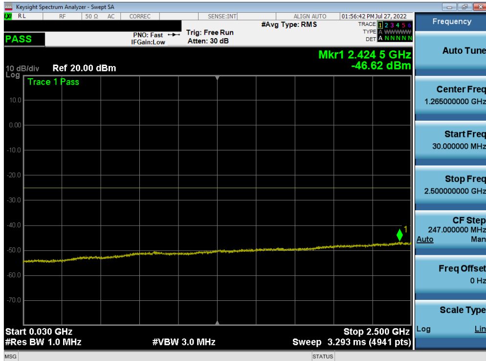
Plot 7-154. Conducted Spurious Plot (LTE Band 7 - 20MHz QPSK - RB Size 1, RB Offset 0 - High Channel)
