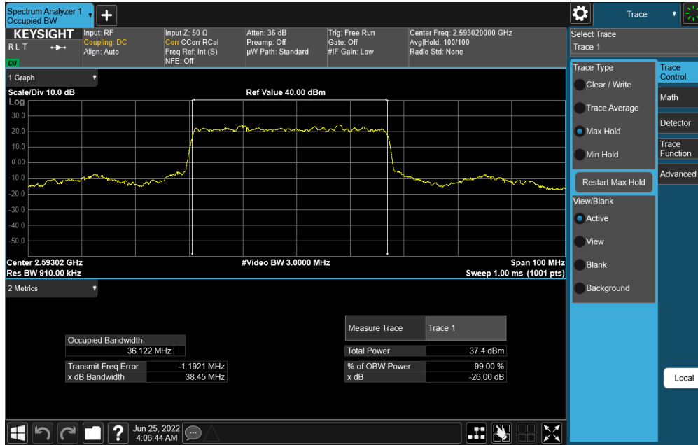
Plot 7-96. Occupied Bandwidth Plot (NR Band n41 - 40MHz DFT-s-OFDM \pi/2 BPSK - Full RB)
