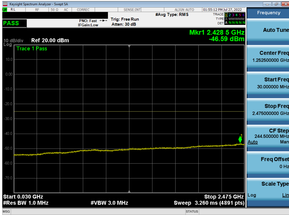
Plot 7-148. Conducted Spurious Plot (LTE Band 7 - 20MHz QPSK - RB Size 1, RB Offset 0 - Low Channel)
