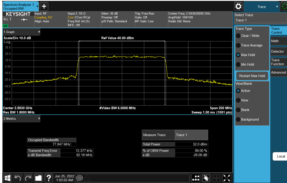
Plot 7-120. Occupied Bandwidth Plot (NR Band n41 - 80MHz CP-OFDM 256-QAM - Full RB)
