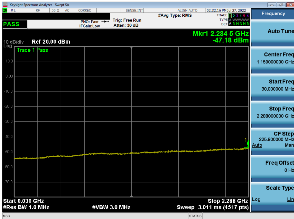
Plot 7-139. Conducted Spurious Plot (LTE Band 30 - 5MHz QPSK - RB Size 1, RB Offset 0 – Low Channel)
