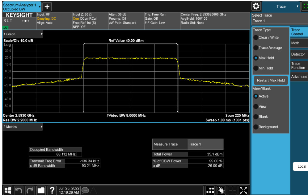
Plot 7-124. Occupied Bandwidth Plot (NR Band n41 - 90MHz CP-OFDM 64-QAM - Full RB)
