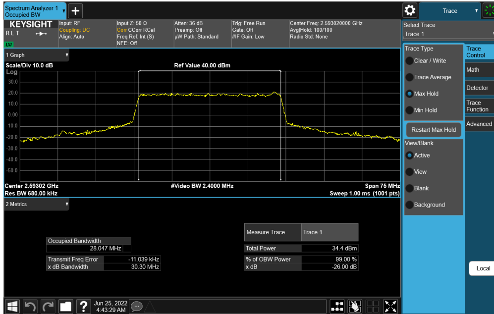
Plot 7-94. Occupied Bandwidth Plot (NR Band n41 - 30MHz CP-OFDM 64-QAM - Full RB)
