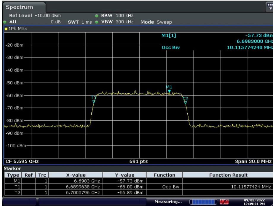
Plot 7-561. AWGN Signal – UNII 7 – 20MHz
