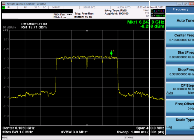
Plot 7-312. Power Spectral Density Plot SDM Antenna 4a (160MHz 802.11ax (UNII Band 5) – Ch. 47, MCS11)
