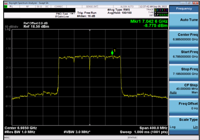
Plot 7-304. Power Spectral Density Plot SDM Antenna 4a (160MHz 802.11ax (UNII Band 8) – Ch. 207, MCS4)
