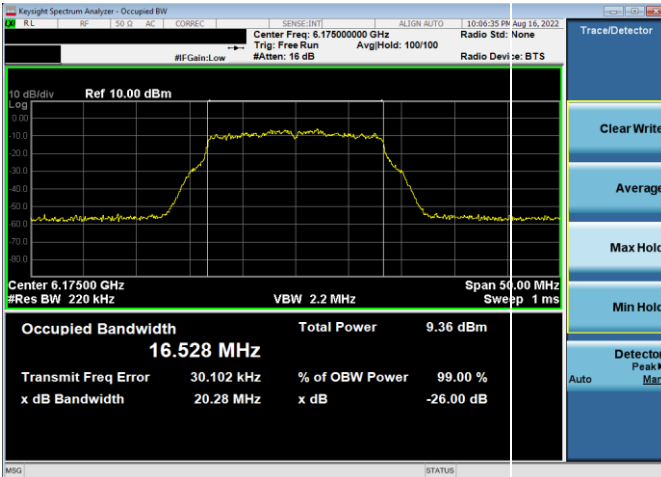
Plot 7-21. 26dB & 99% Bandwidth Plot Antenna 5b (20MHz 802.11a (UNII Band 5) – Ch. 45, 24Mbps)
