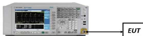
Figure 7-5. Radiated Measurement Setup
