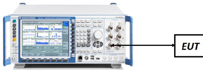
Figure 7-4. Conducted Power Measurement Setup
