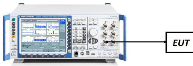
Figure 7-5. ERP/EIRP Measurement Setup
