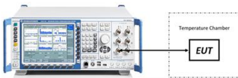
Figure 7-8. Test Instrument & Measurement Setup
