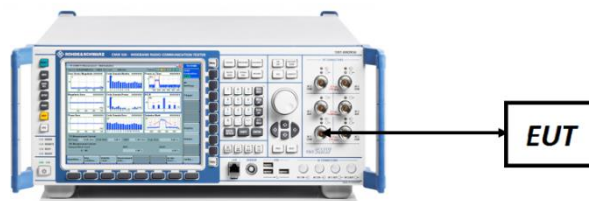
Figure 7-7. ERP/EIRP Measurement Setup
