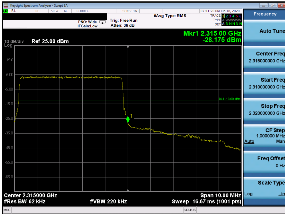
Plot 7-303. Upper Band Edge Plot (Band 30 - 5.0MHz QPSK - Full RB Configuration)
