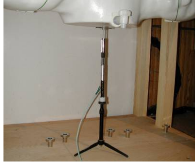
Figure 9-2 System Verification Setup Photo
