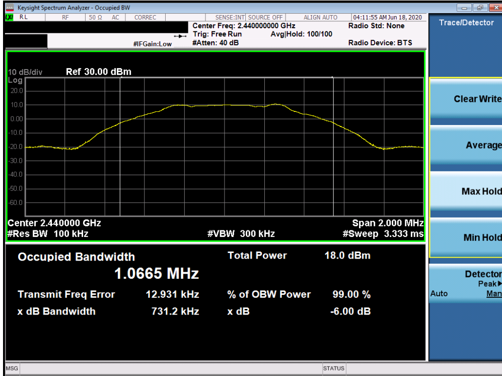
Plot 7-5. 6dB Bandwidth Plot (Bluetooth (LE), 1Mbps, iPA – Ch. 19)
