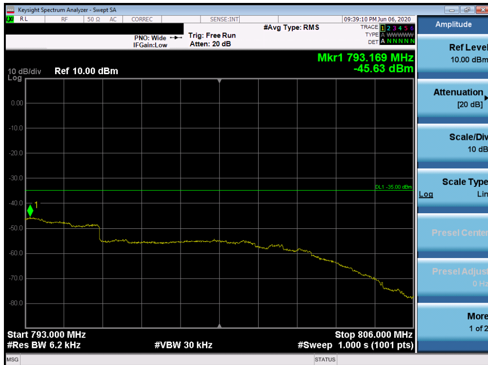
Plot 7-217. Higher Emission Mask Edge Plot (Band 13 - 10.0MHz QPSK - Full RB Configuration)
