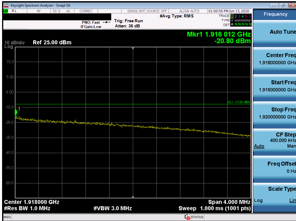
Plot 7-297. Upper Extended Band Edge Plot (Band 25 - 10.0MHz QPSK - Full RB Configuration)
