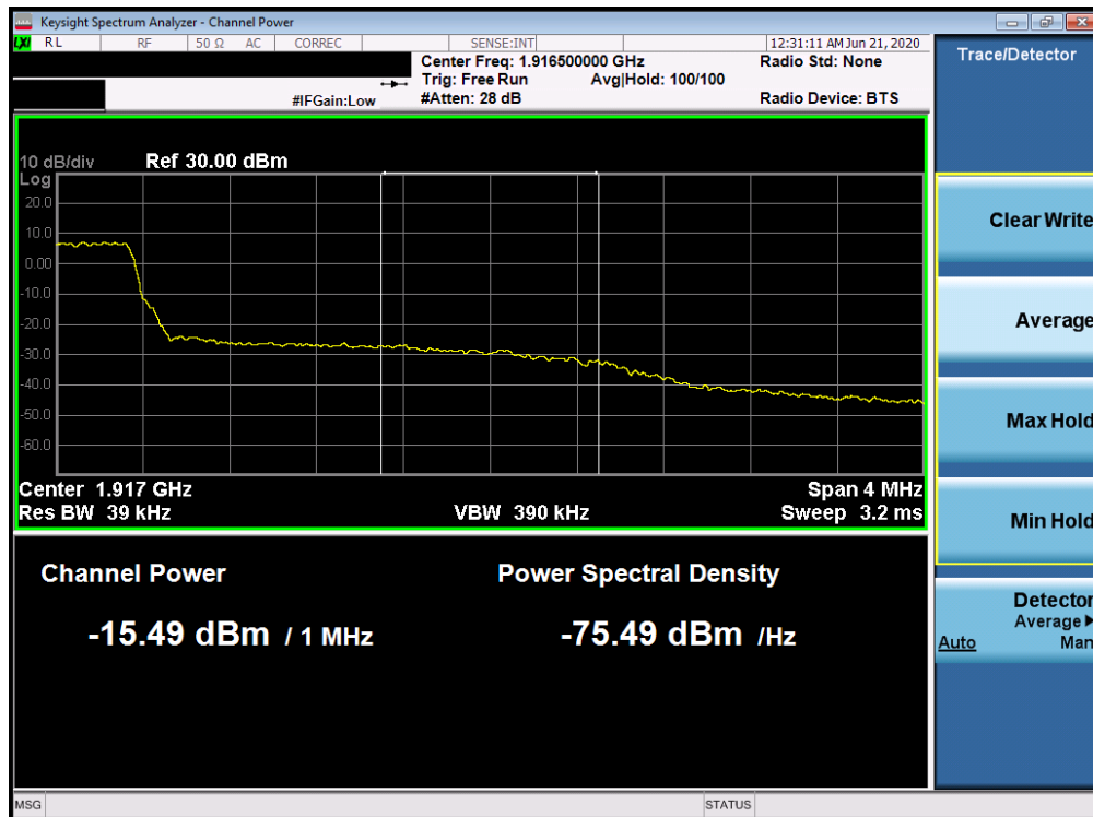
Plot 7-289. Upper Extended Band Edge Plot (Band 25 - 3.0MHz QPSK - Full RB Configuration)
