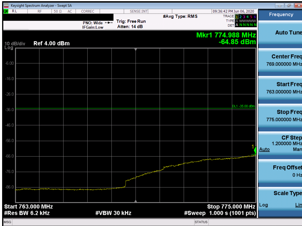
Plot 7-215. Lower Emission Mask Edge Plot (Band 13 - 10.0MHz QPSK - Full RB Configuration)
