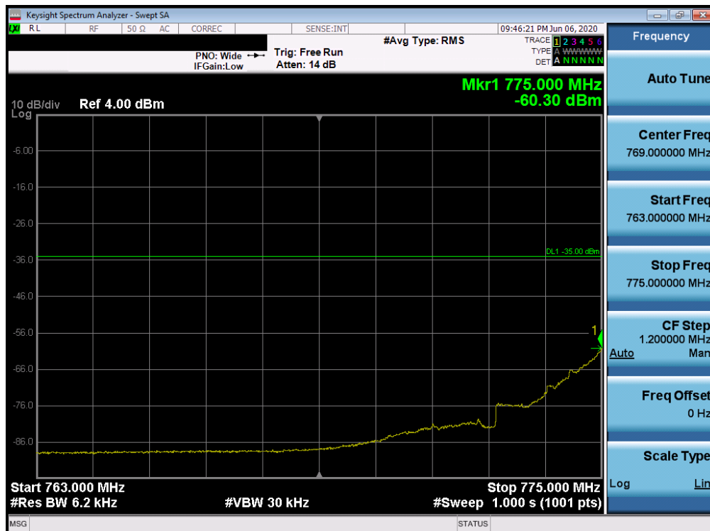
Plot 7-211. Lower Emission Mask Edge Plot (Band 13 - 5.0MHz QPSK - Full RB Configuration)
