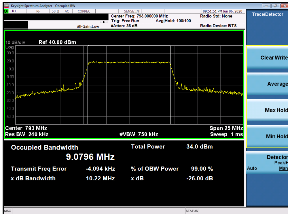
Plot 7-14. Occupied Bandwidth Plot (Band 14 - 10MHz 16-QAM - Full RB Configuration)
