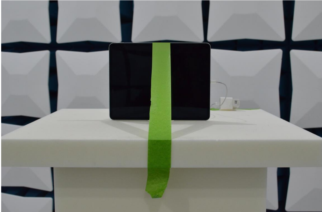
Figure 7: 1-18GHz Test Setup (Front View)
