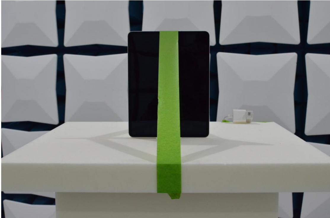
Figure 9: 1-18GHz Test Setup (Front View)
