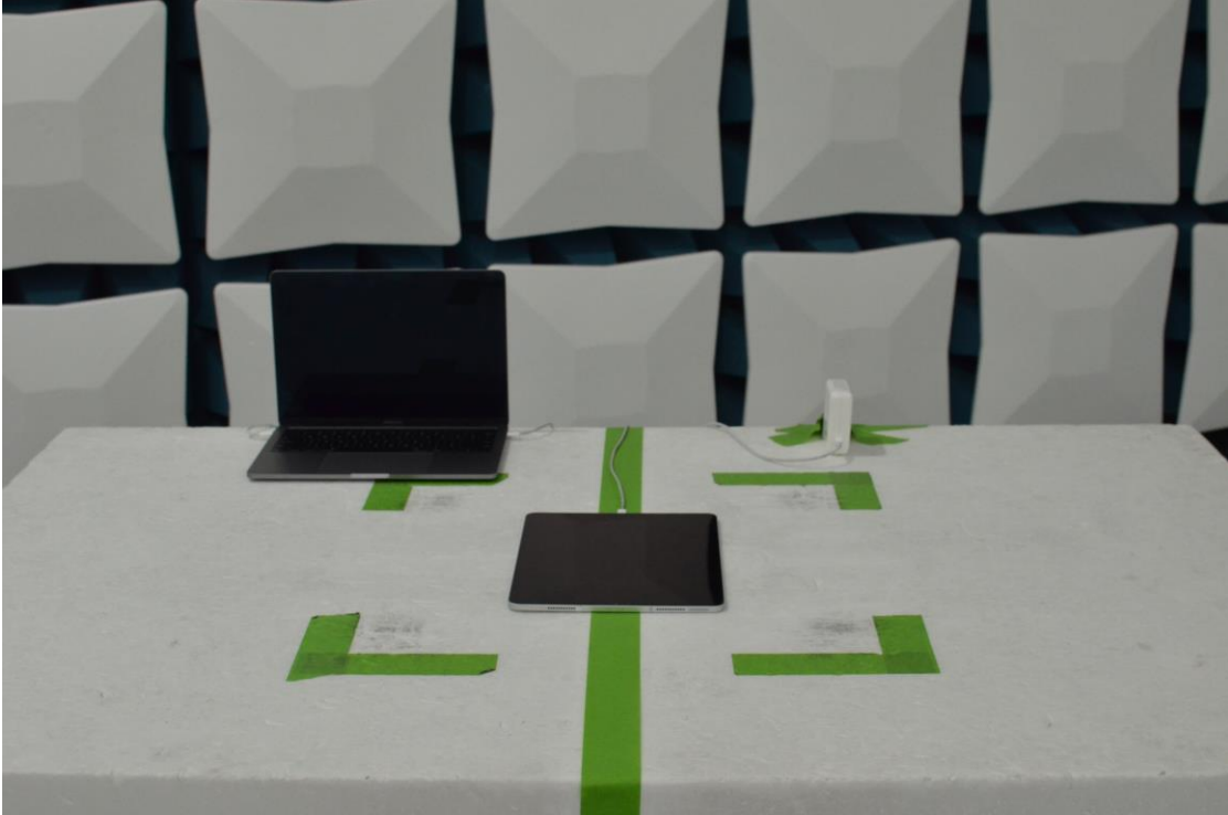
Figure 17: 30MHz-1GHz Test Setup (Front View)
