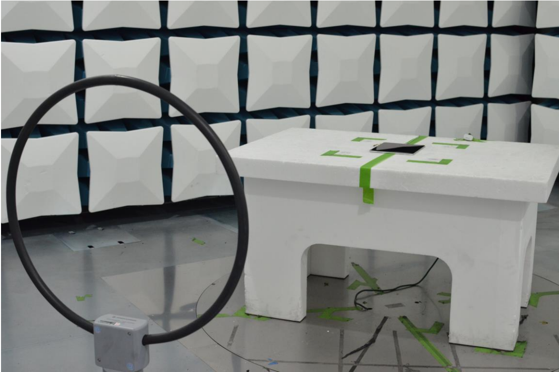
Figure 23: 9kHz-30MHz Test Setup (Front View)
