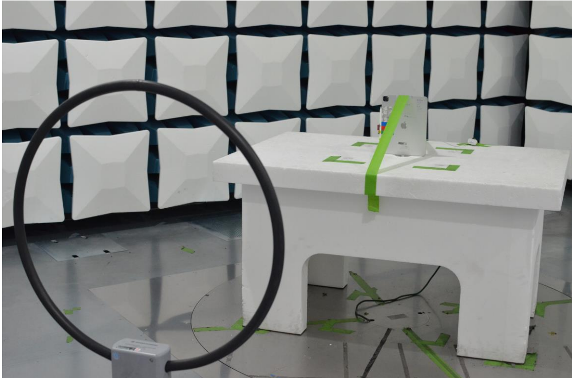
Figure 25: 9kHz-30MHz Test Setup (Front View)
