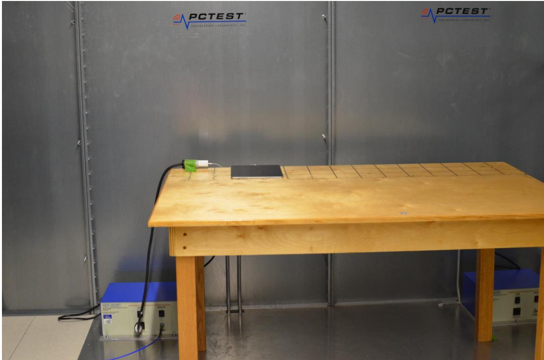
Figure 1: AC Line Conducted Emissions (Front View)
