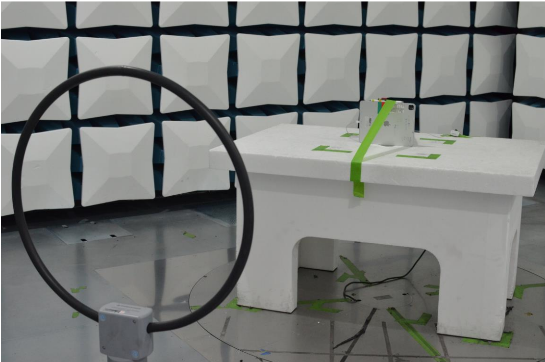
Figure 24: 9kHz-30MHz Test Setup (Front View)
