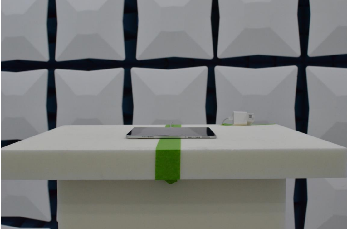
Figure 5: 1-18GHz Test Setup (Front View)
