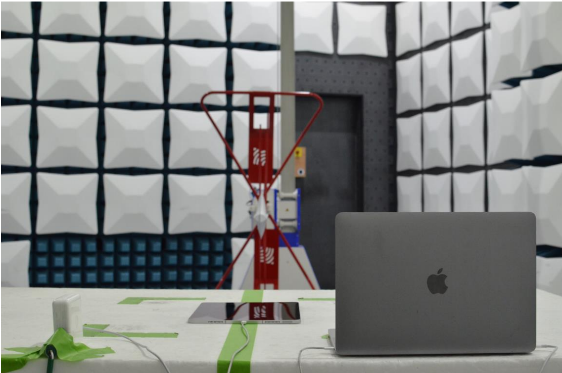
Figure 18: 30MHz-1GHz Test Setup (Rear View)
