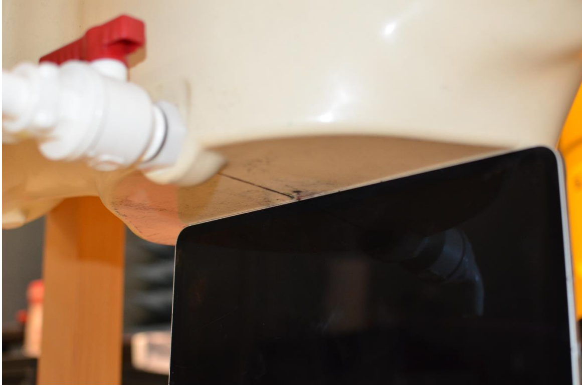
SAR Test Setup Photo 9: Left Edge at 0.0 cm – Ant 2a/2b/1
