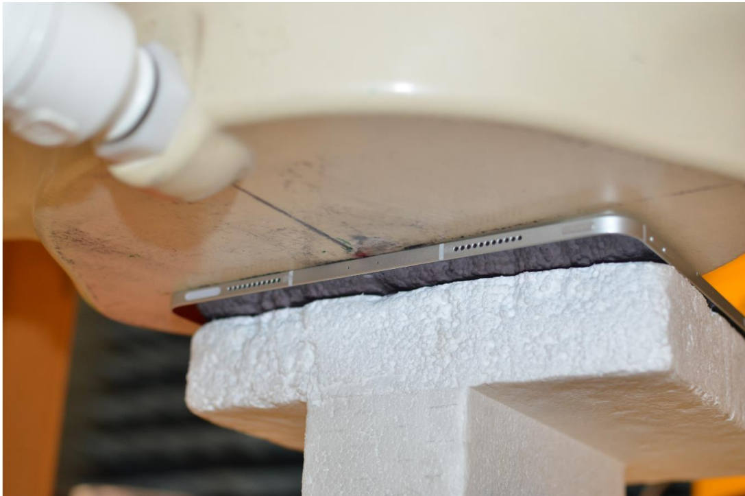
SAR Test Setup Photo 1: Back Side at 0.0 cm – Ant 4a/4b/3
