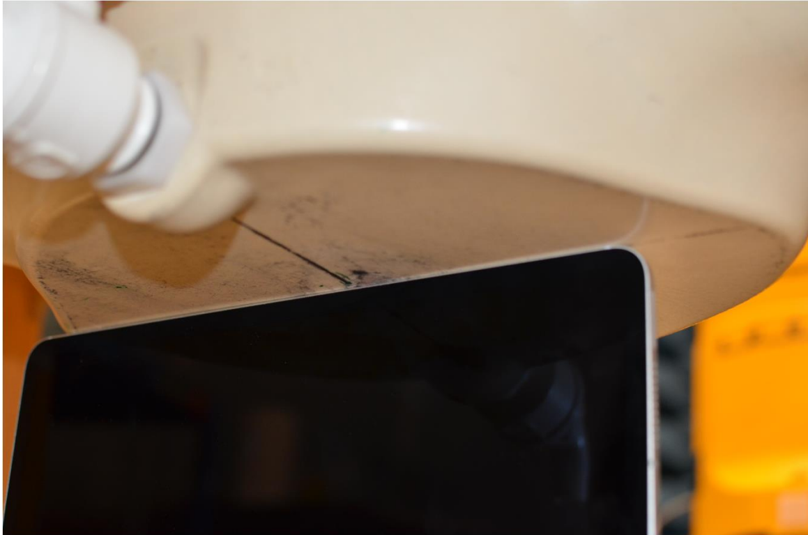
SAR Test Setup Photo 7: Right Edge at 0.0 cm – Ant 2a/2b/1
