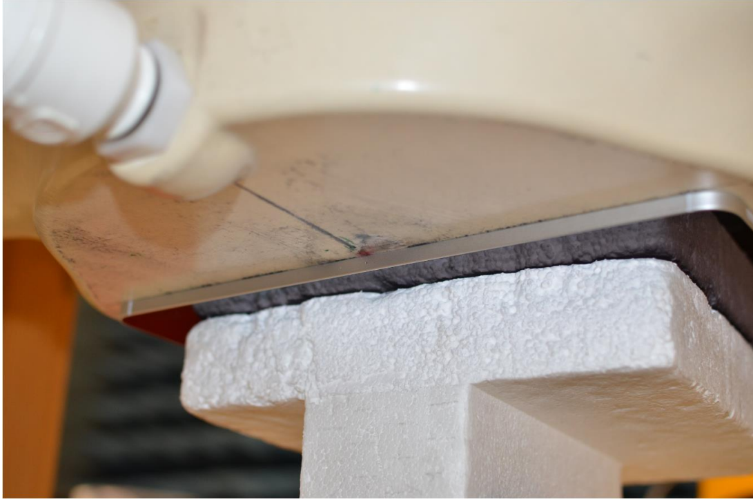
SAR Test Setup Photo 3: Back Side at 0.0 cm – Ant 5b
