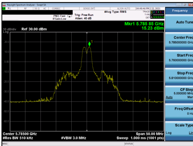
Plot 7-291. PSD CDD Antenna 5T (20MHz BW 11ax Index 4 – RU26 – Ch.157)
