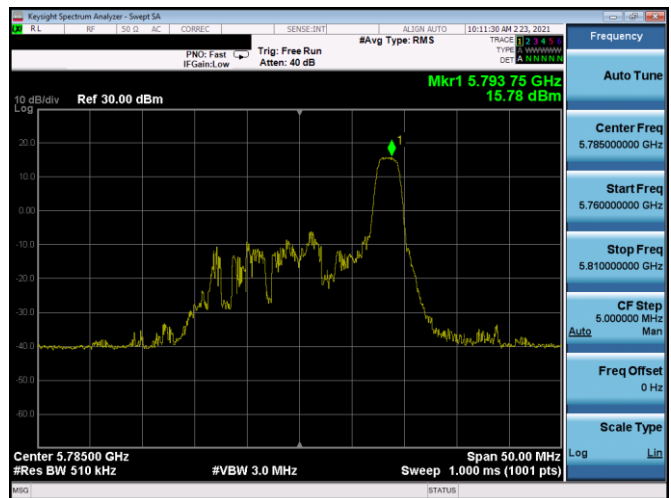
Plot 7-294. PSD CDD Antenna 5B (20MHz BW 11ax Index 8– RU26 – Ch.157)
