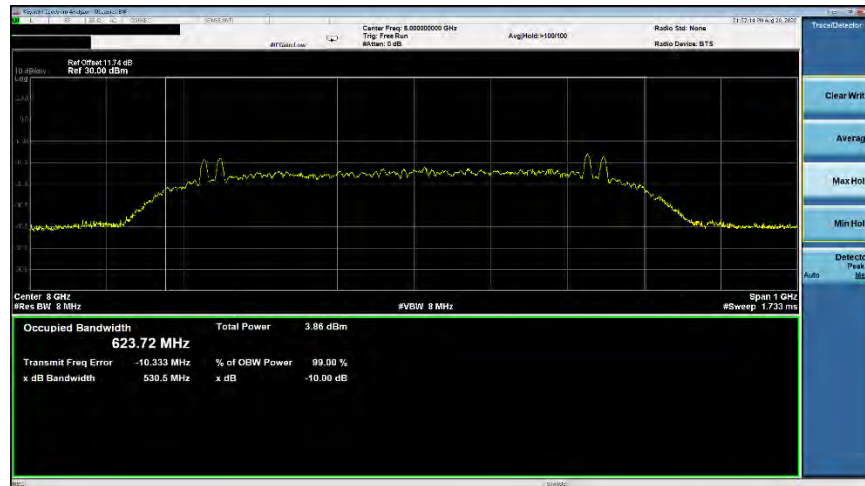
Plot 7-34. ISED Occupied Bandwidth (Ch. 9, Config 1/Payload 45)
