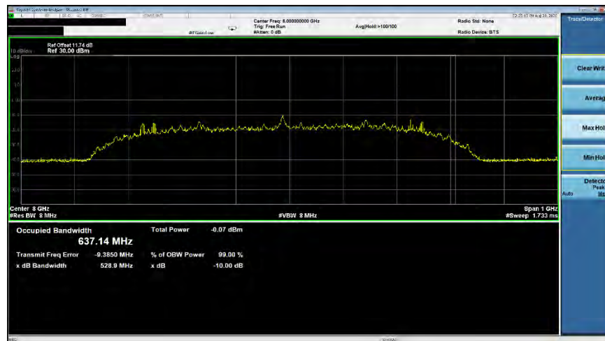
Plot 7-38. ISED Occupied Bandwidth (Ch. 9, Config 3/Payload 125)
