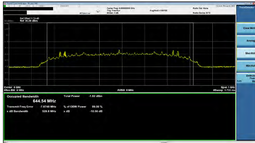
Plot 7-37. ISED Occupied Bandwidth (Ch. 9, Config 2/Payload 125)
