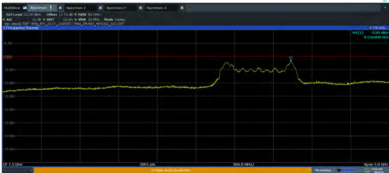
Plot 7-59. Peak Radiated Power (Ch. 9, Config 4/Payload 0)
