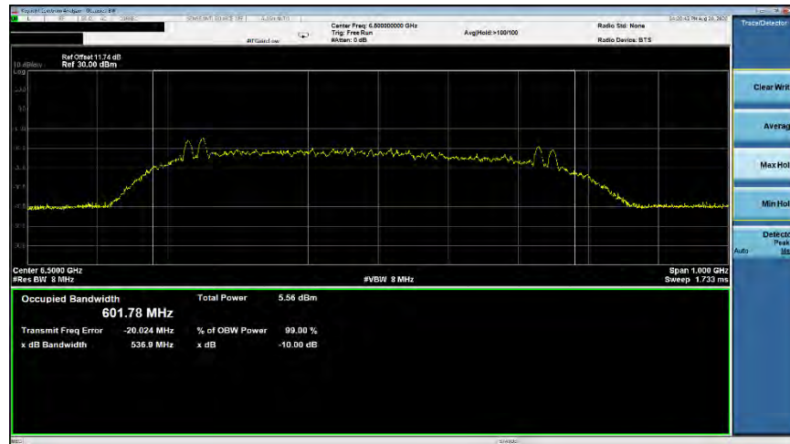
Plot 7-22. ISCED Occupied Bandwidth (Ch. 5, Config 0/Payload 65)
