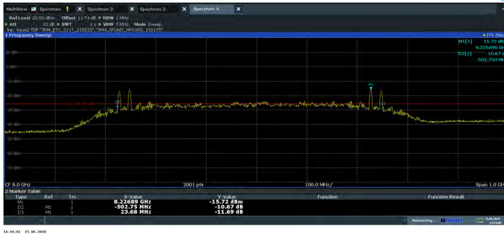
Plot 7-15. 10dBc Bandwidth (Ch. 9, Config 1/Payload 85)
