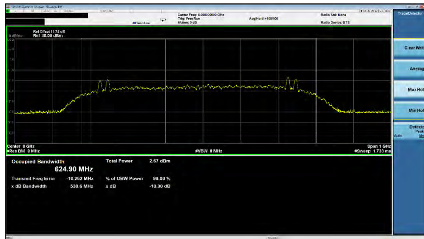
Plot 7-35. ISED Occupied Bandwidth (Ch. 9, Config 1/Payload 85)
