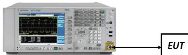
Figure 7-3. Test Instrument & Measurement Setup
