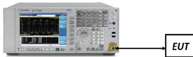
Figure 7-4. Test Instrument & Measurement Setup
