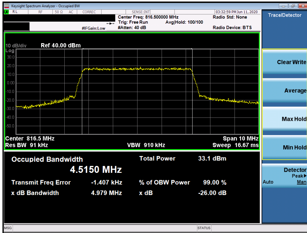
Plot 7-3. Occupied Bandwidth Plot (LTE Band 26 - 5MHz QPSK - Full RB Configuration)
