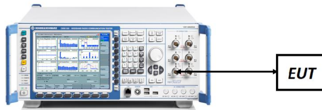
Figure 7-4. Conducted Power Measurement Setup
