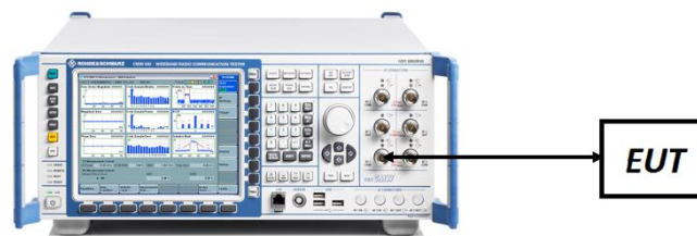
Figure 7-5. ERP/EIRP Measurement Setup
