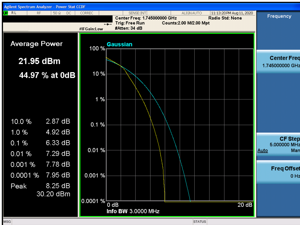
Plot 7-229. PAR Plot (Band 66 - 3.0MHz 16-QAM - Full RB Configuration)
