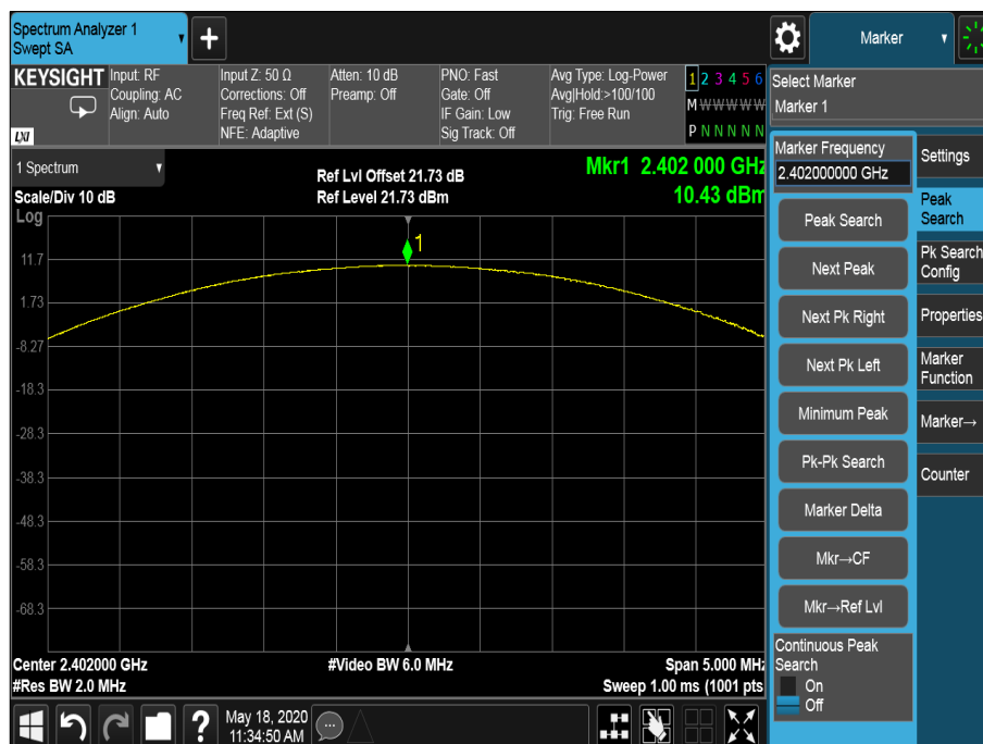
Figure 12 - 2402 MHz - Maximum Output Power, 8-DPSK
