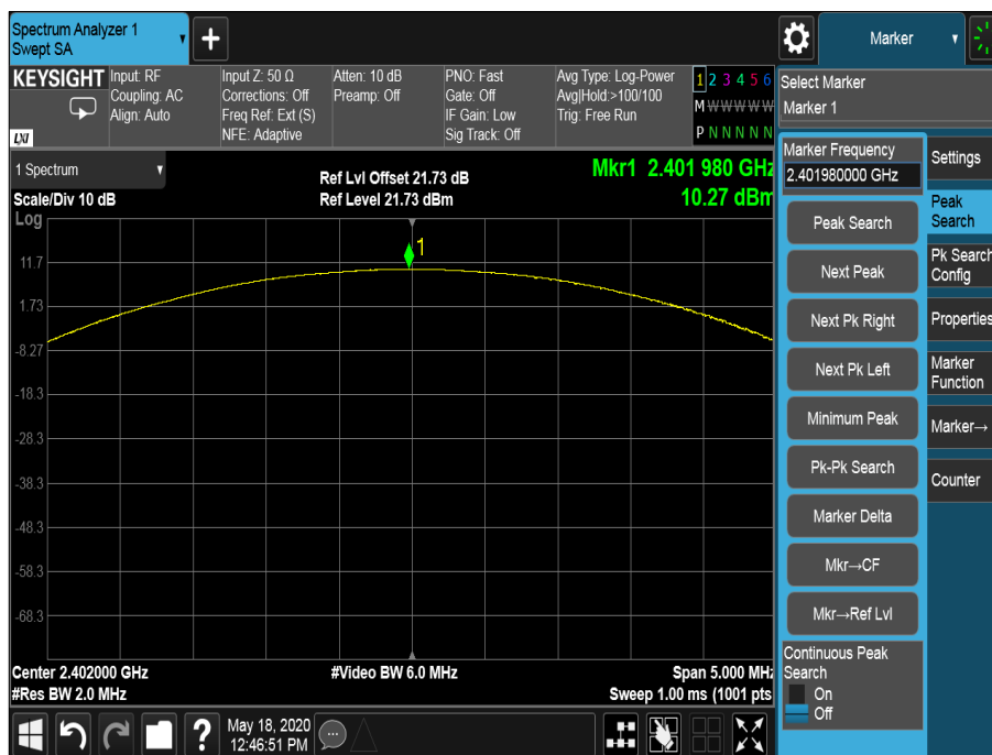
Figure 3 - 2402 MHz - Maximum Output Power, 8-DPSK
