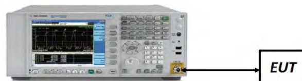
Figure 7-1. Test Instrument & Measurement Setup
