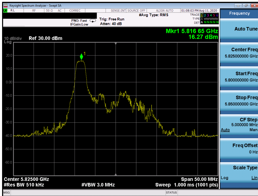
Plot 7-1140. Power Spectral Density Plot CDD Diversity Antenna 1b (20MHz BW 802.11ax Index 0 – RU26 (UNII Band 3) – Ch. 165)
