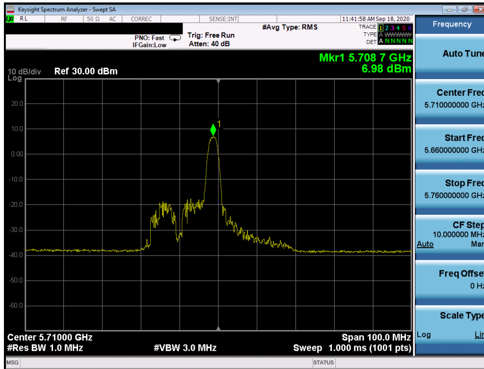
Plot 7-1097. Power Spectral Density Plot CDD Diversity Antenna 2b (40MHz BW 802.11ax Index 8 – RU26 (UNII Band 2C) – Ch. 142)
