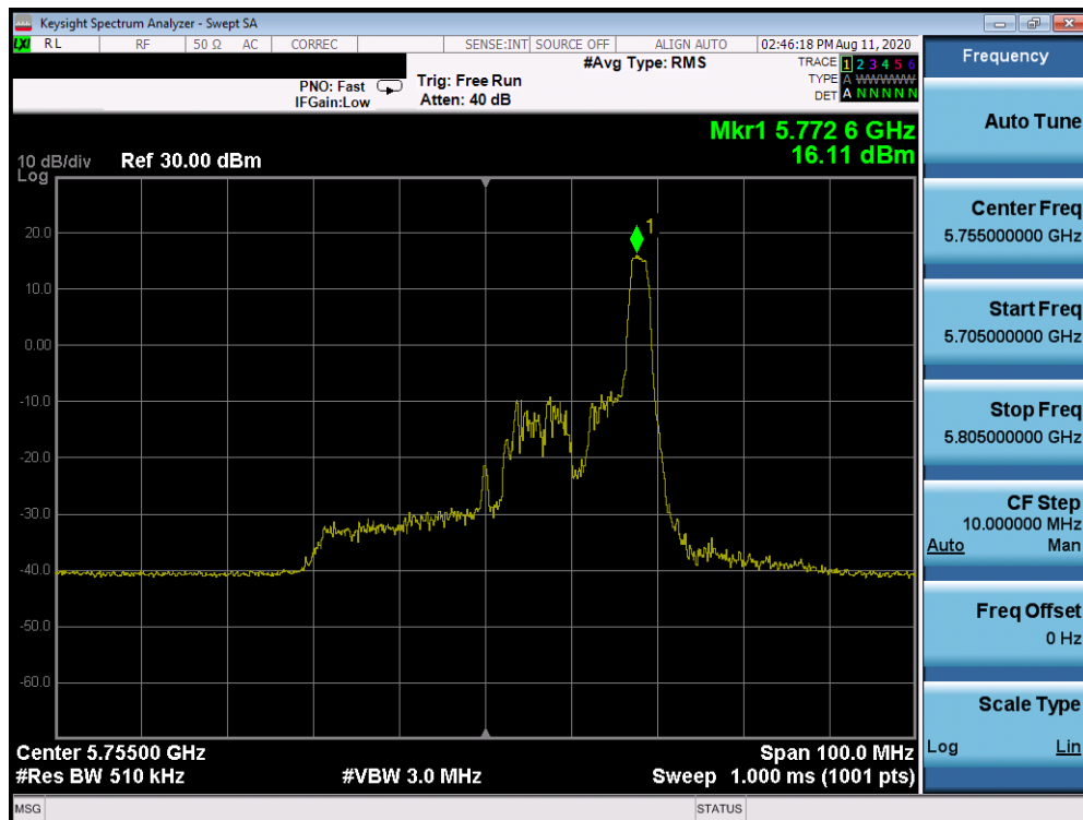
Plot 7-1156. Power Spectral Density Plot CDD Diversity Antenna 1b (40MHz BW 802.11ax Index 17 – RU26 (UNII Band 3) – Ch. 151)
