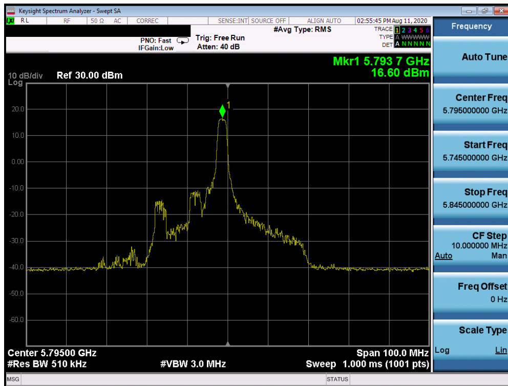
Plot 7-1160. Power Spectral Density Plot CDD Diversity Antenna 1b (40MHz BW 802.11ax Index 8 – RU26 (UNII Band 3) – Ch. 159)
