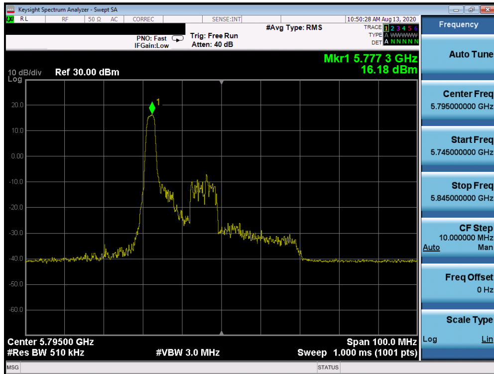
Plot 7-1157. Power Spectral Density Plot CDD Diversity Antenna 2b (40MHz BW 802.11ax Index 0 – RU26 (UNII Band 3) – Ch. 159)
