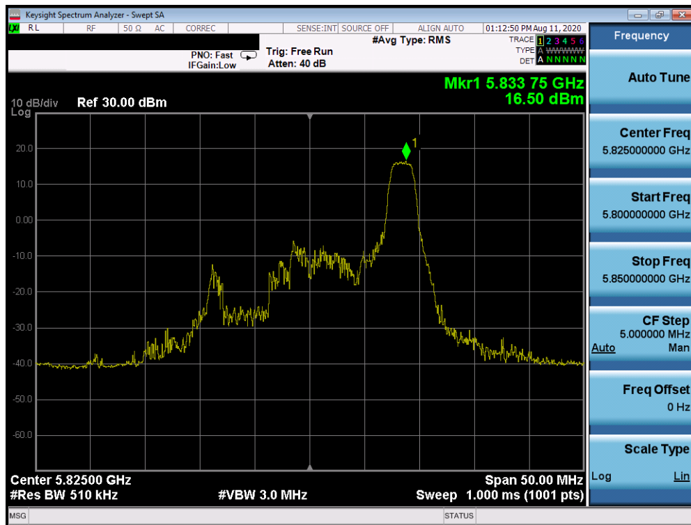
Plot 7-1144. Power Spectral Density Plot CDD Diversity Antenna 1b (20MHz BW 802.11ax Index 8 – RU26 (UNII Band 3) – Ch. 165)
