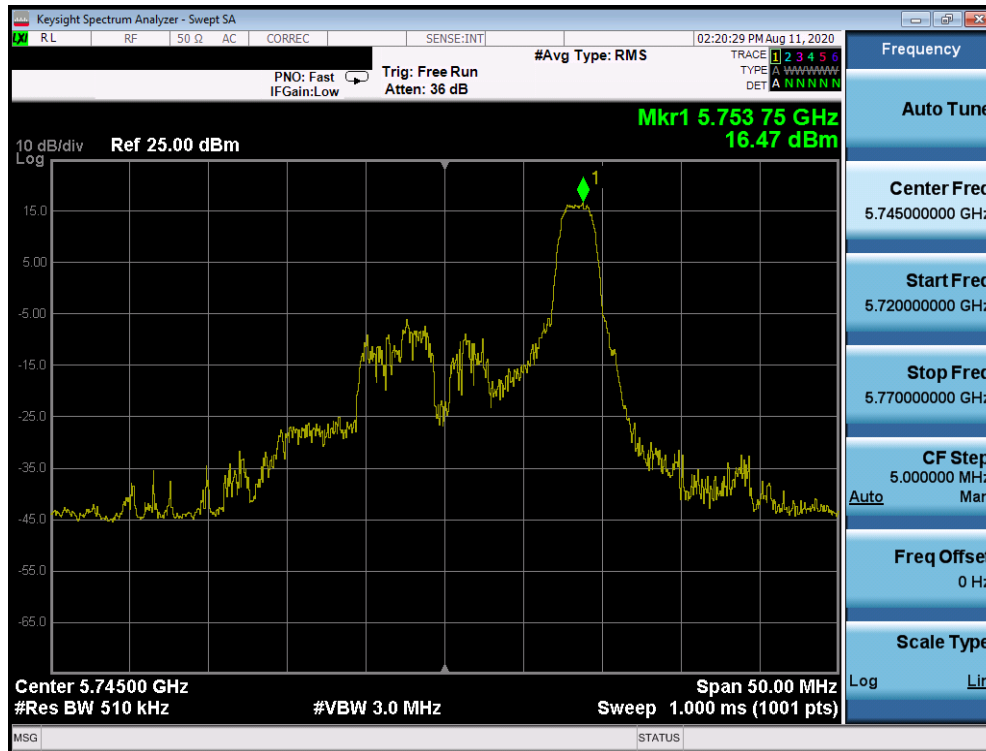
Plot 7-1131. Power Spectral Density Plot CDD Diversity Antenna 2b (20MHz BW 802.11ax Index 8 – RU26 (UNII Band 3) – Ch. 149)
