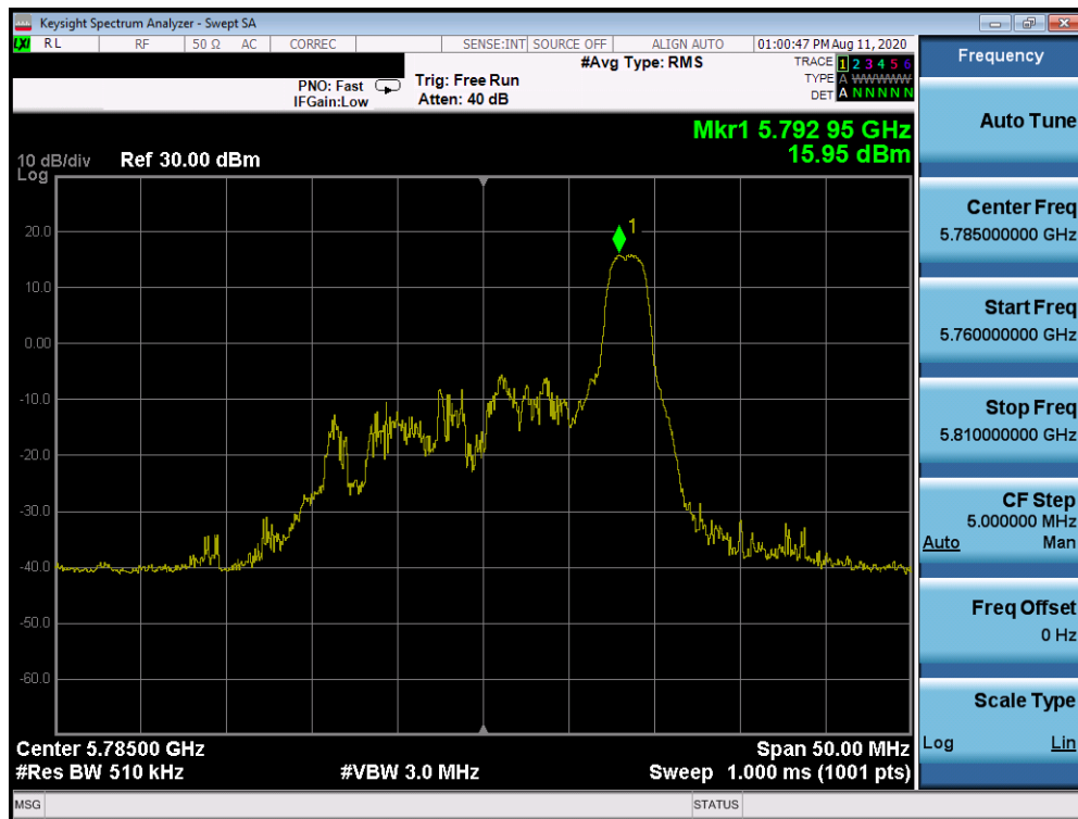
Plot 7-1138. Power Spectral Density Plot CDD Diversity Antenna 1b (20MHz BW 802.11ax Index 8- RU26 (UNII Band 3) – Ch. 157)
