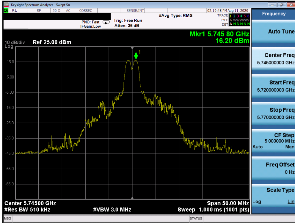
Plot 7-869. Power Spectral Density Plot CDD Primary Antenna 2b (20MHz BW 802.11ax Index 4 – RU26 (UNII Band 3) – Ch. 149)
