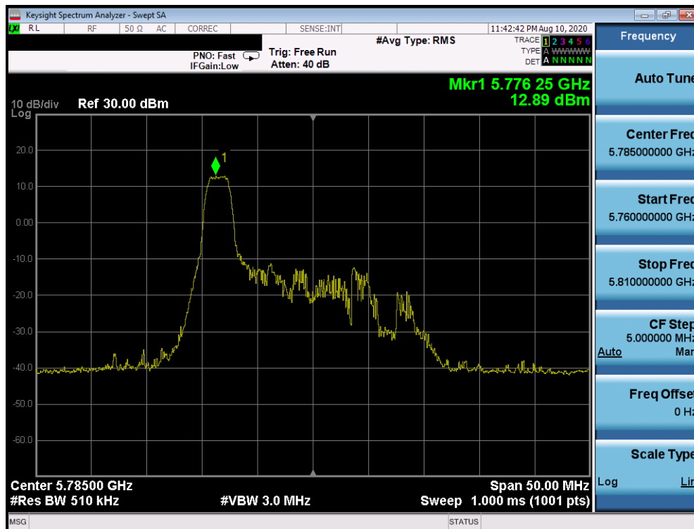
Plot 7-874. Power Spectral Density Plot CDD Primary Antenna 2a (20MHz BW 802.11ax Index 0 – RU26 (UNII Band 3) – Ch. 157)
