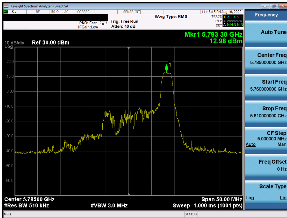
Plot 7-878. Power Spectral Density Plot CDD Primary Antenna 2a (20MHz BW 802.11ax Index 8– RU26 (UNII Band 3) – Ch. 157)
