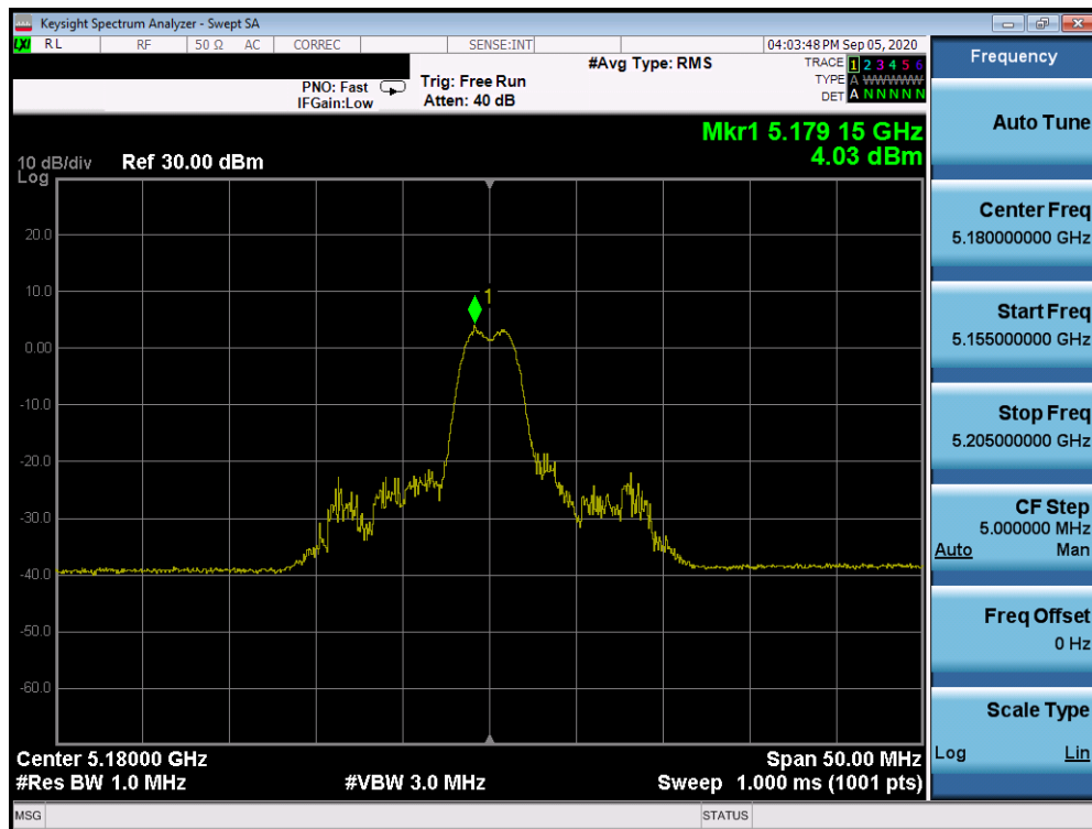
Plot 7-680. ISED Power Spectral Density Plot Antenna 1b (20MHz BW 802.11ax Index 4 – RU26 (UNII Band 1) – Ch. 36)
