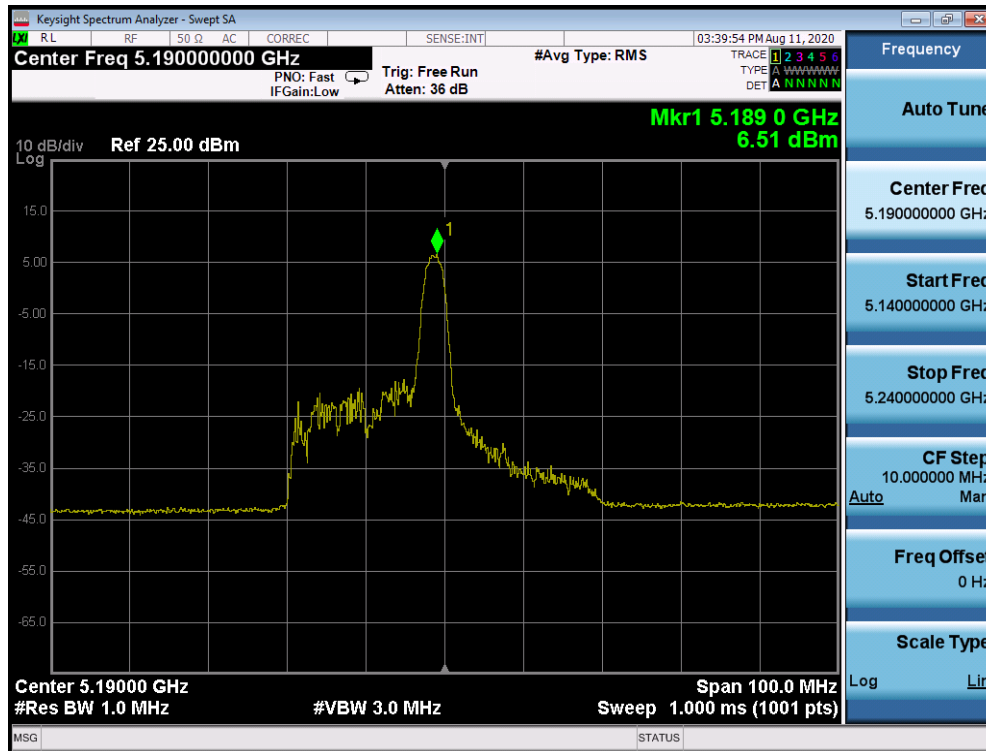
Plot 7-729. Power Spectral Density Plot CDD Primary Antenna 2b (40MHz BW 802.11ax Index 8 – RU26 (UNII Band 1) – Ch. 38)
