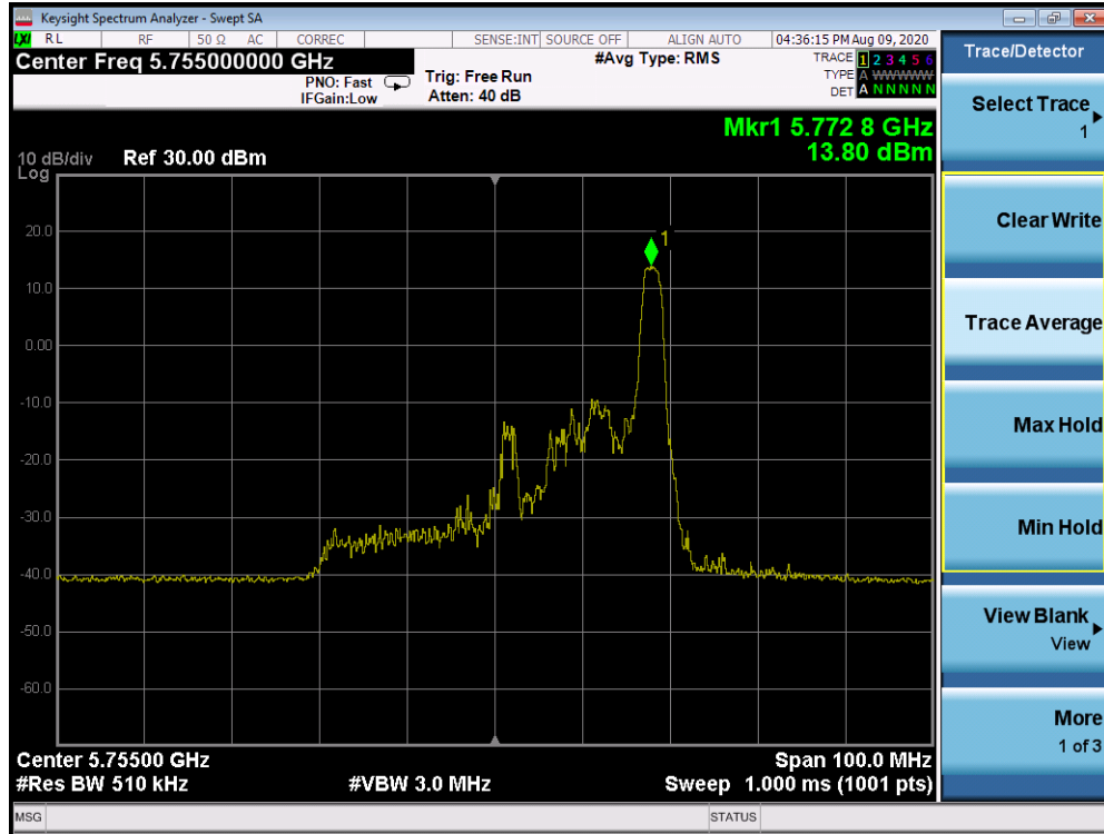
Plot 7-669. Power Spectral Density Plot Antenna 1b (40MHz BW 802.11ax Index 17 – RU26 (UNII Band 3) – Ch. 151)
