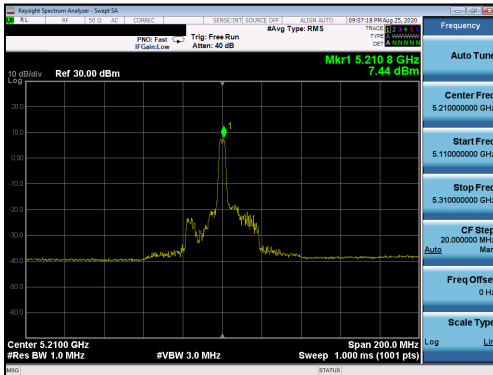
Plot 7-464. Power Spectral Density Plot Antenna 2a (80MHz BW 802.11ax Index 18 – RU26 (UNII Band 1) – Ch. 42)
