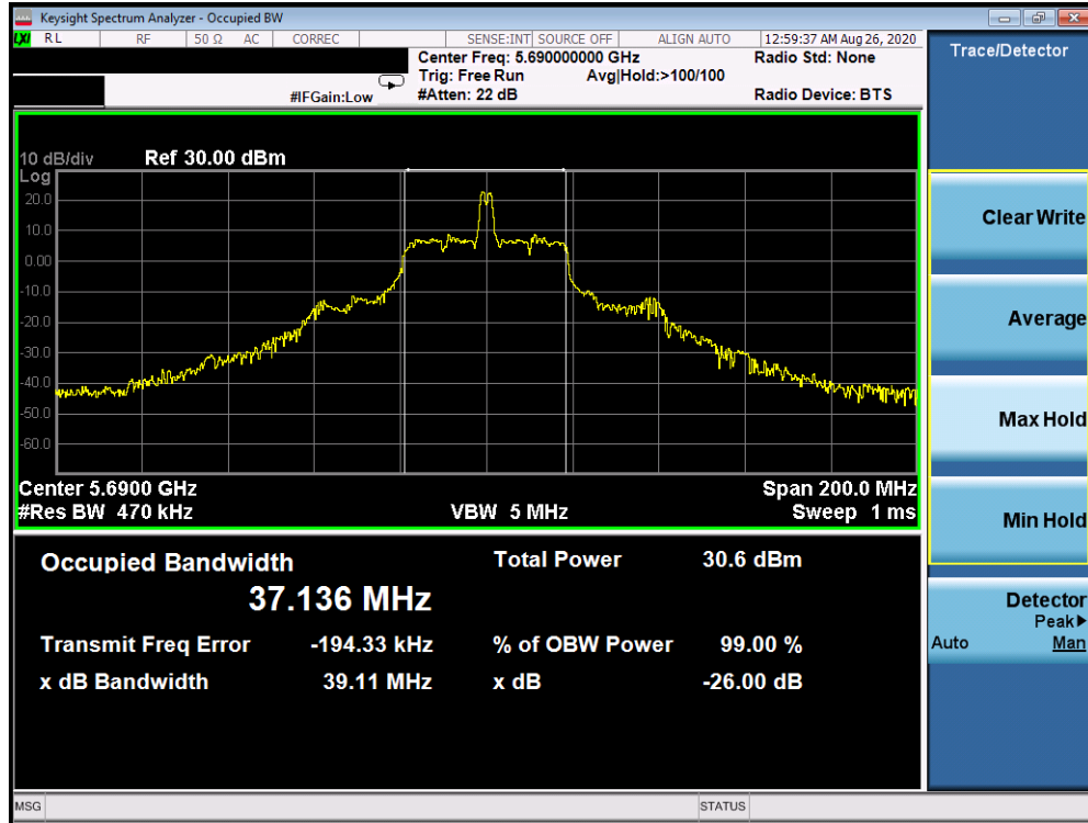
Plot 7-237. 26dB Bandwidth Plot Antenna 1b (80MHz BW 802.11ax Index 18 – RU26 (UNII Band 2C) – Ch. 138)
