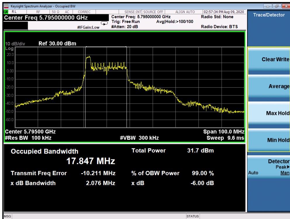
Plot 7-256. 6dB Bandwidth Plot Antenna 2b (40MHz BW 802.11ax Index 0 – RU26 (UNII Band 3) – Ch. 159)
