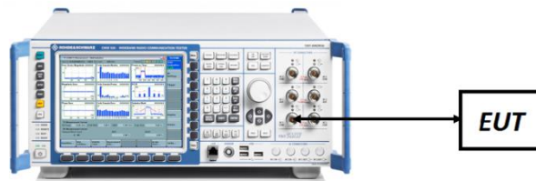
Figure 7-7. ERP/EIRP Measurement Setup
