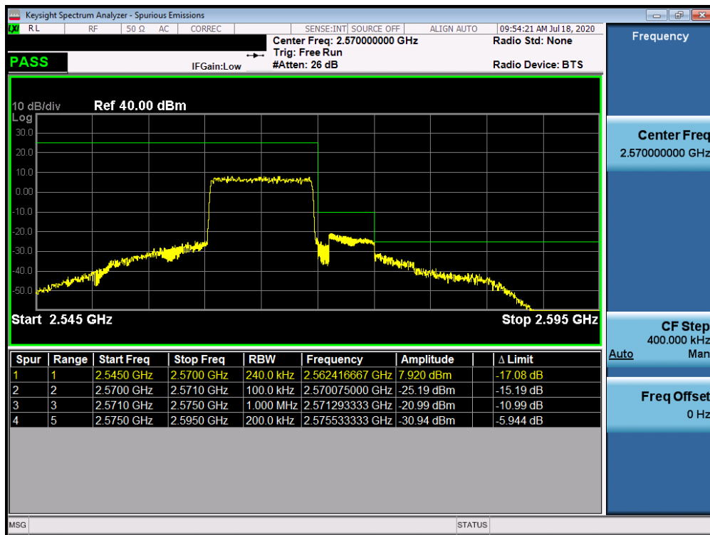
Plot 7-341. Upper ACP Plot (Band 7 - 10.0MHz QPSK - Full RB Configuration)
