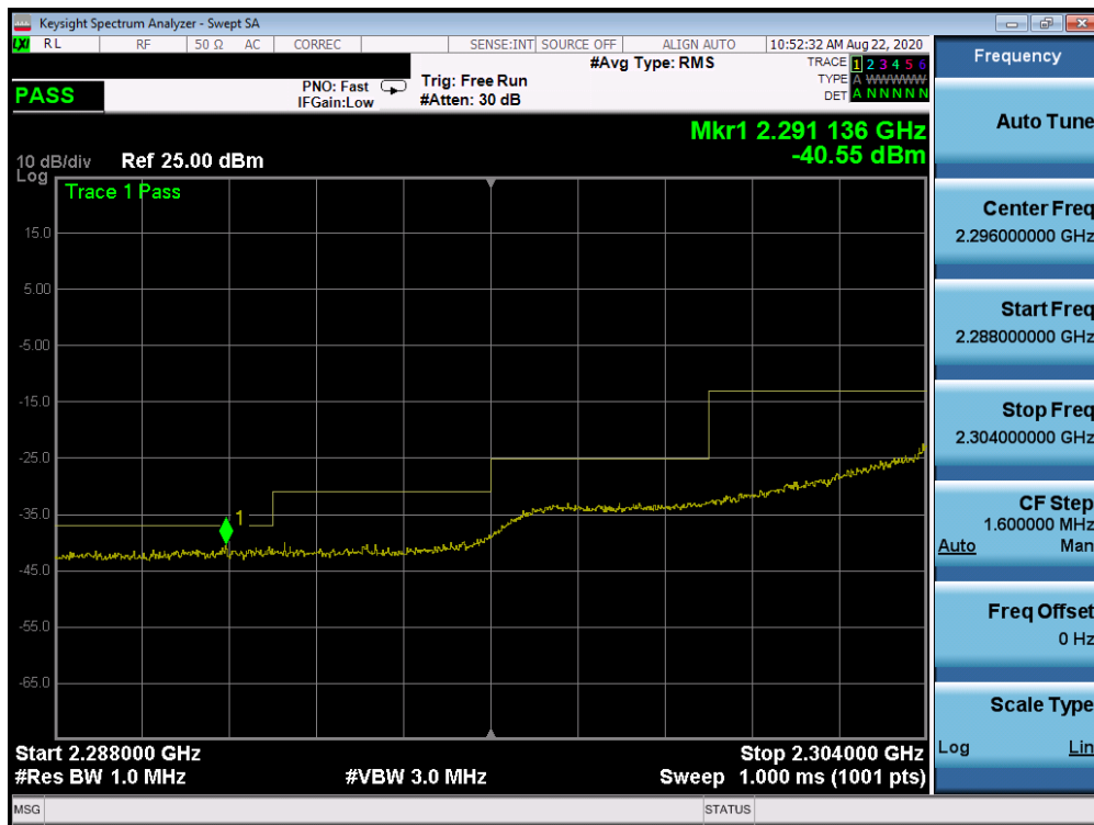
Plot 7-335. Lower Extended Band Edge Plot (Band 30 - 10.0MHz QPSK - Full RB Configuration)
