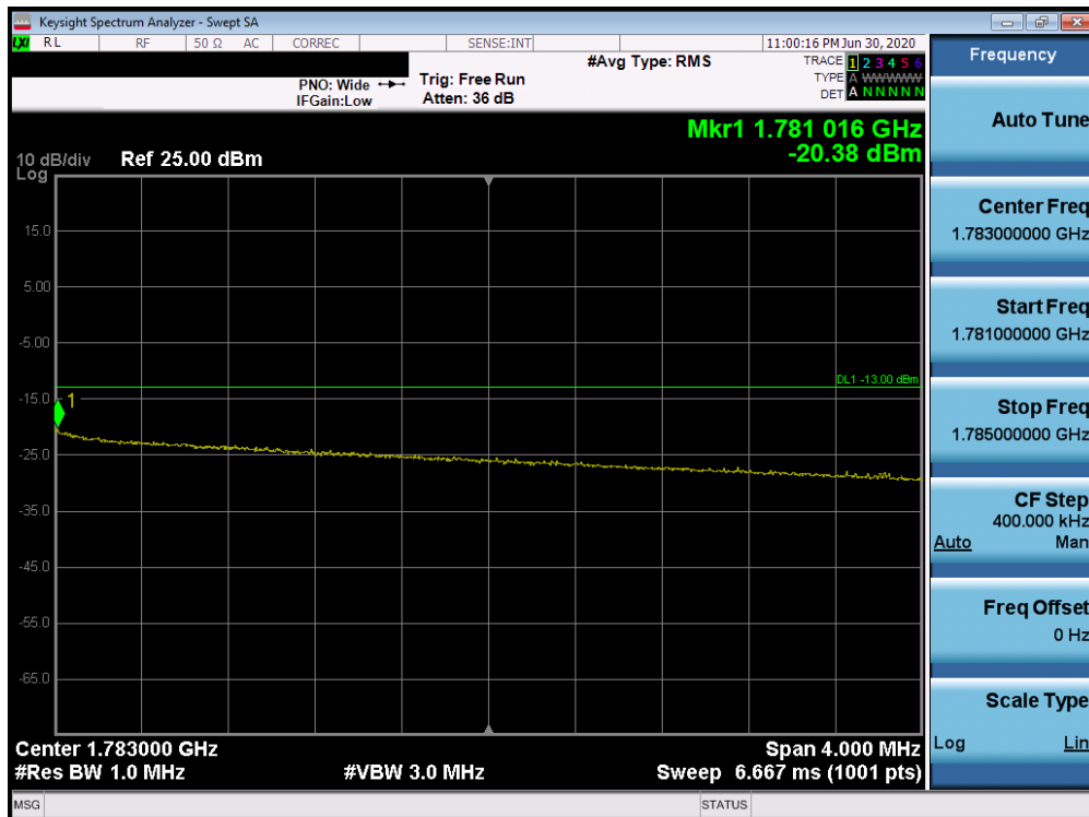
Plot 7-249. Upper Extended Band Edge Plot (Band 66 - 10.0MHz QPSK - Full RB Configuration)
