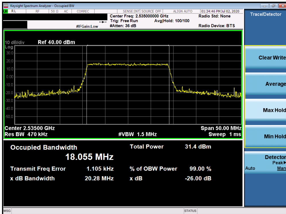
Plot 7-96. Occupied Bandwidth Plot (Band 7 - 20.0MHz 64-QAM - Full RB Configuration)
