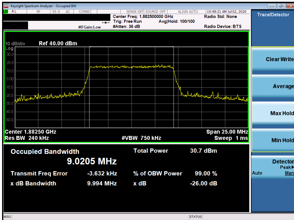
Plot 7-72. Occupied Bandwidth Plot (Band 25/2 - 10.0MHz 64-QAM - Full RB Configuration)
