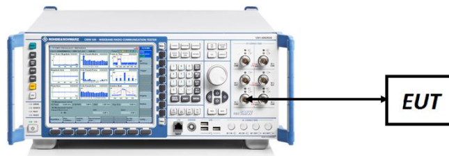
Figure 7-4. ERP/EIRP Measurement Setup
