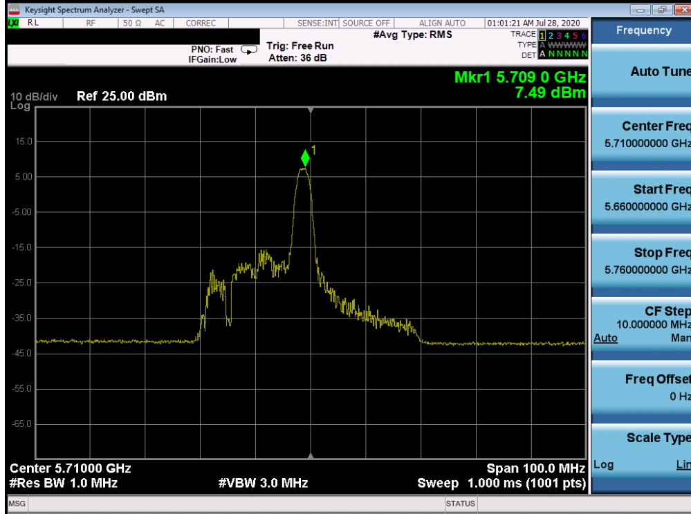
Plot 7-599. Power Spectral Density Plot CDD ANT WF8 (40MHz BW 802.11ax Index 8 – RU26 (UNII Band 2C) – Ch. 142)
