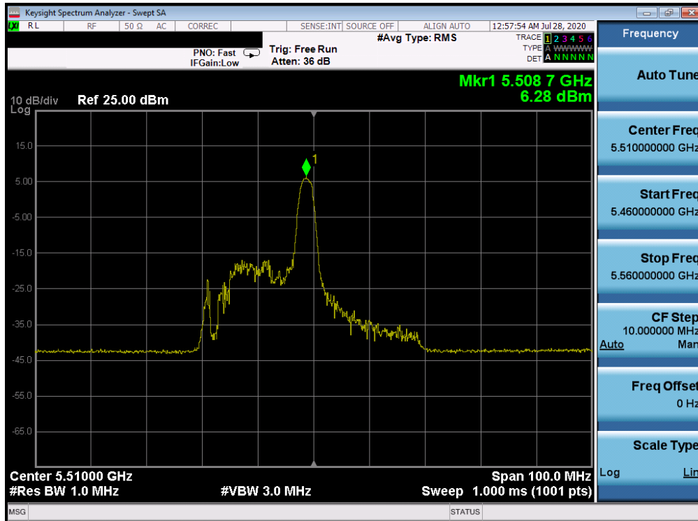
Plot 7-587. Power Spectral Density Plot CDD ANT WF8 (40MHz BW 802.11ax Index 8 – RU26 (UNII Band 2C) – Ch. 102)
