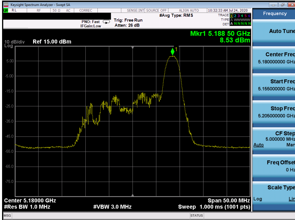
Plot 7-339. Power Spectral Density Plot ANT WF7a (20MHz BW 802.11ax Index 8 – RU26 (UNII Band 1) – Ch. 36)
