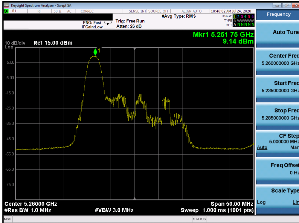
Plot 7-361. Power Spectral Density Plot ANT WF7a (20MHz BW 802.11ax Index 0 – RU26 (UNII Band 2A) – Ch. 52)
