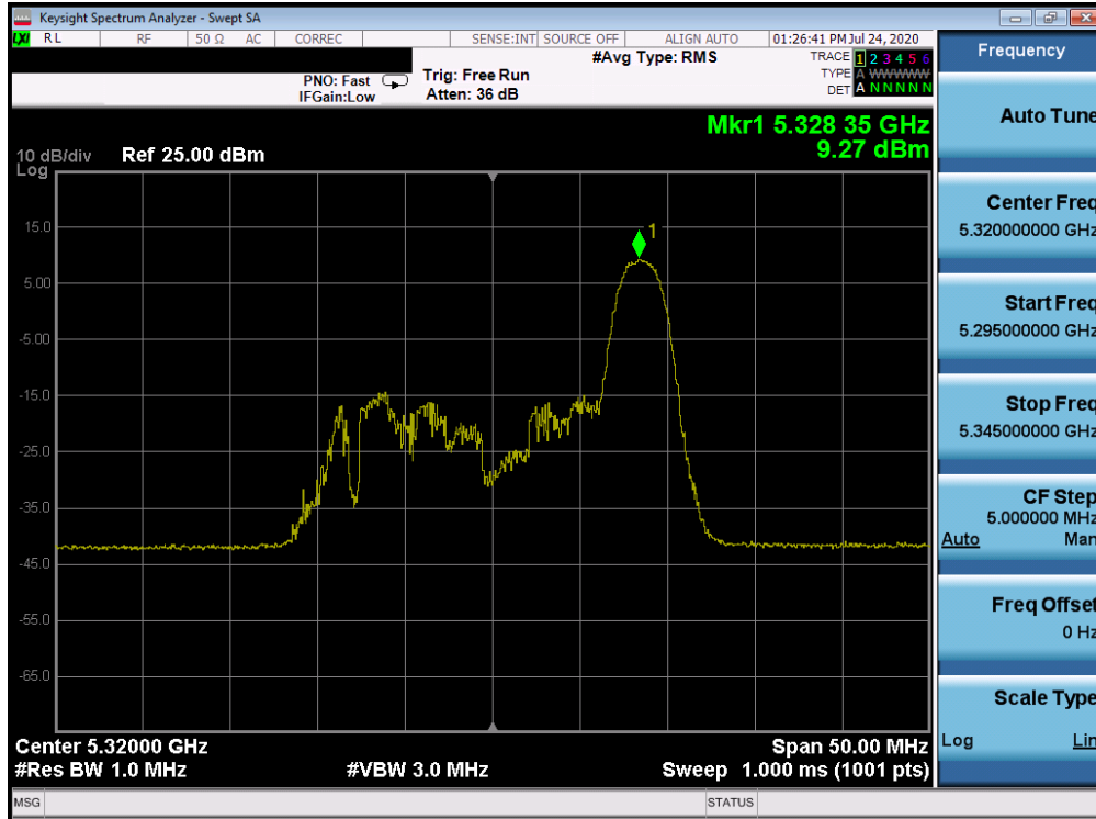
Plot 7-369. Power Spectral Density Plot ANT WF7a (20MHz BW 802.11ax Index 8 – RU26 (UNII Band 2A) – Ch. 64)
