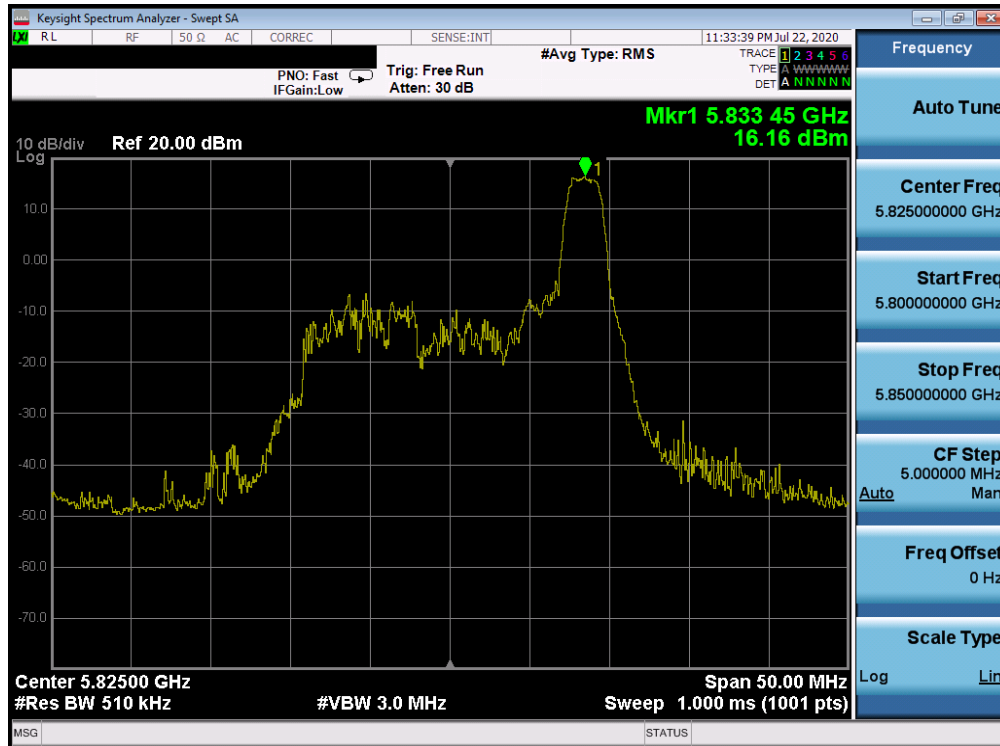
Plot 7-297. Power Spectral Density Plot ANT WF8 (20MHz BW 802.11ax Index 8 – RU26 (UNII Band 3) – Ch. 165)
