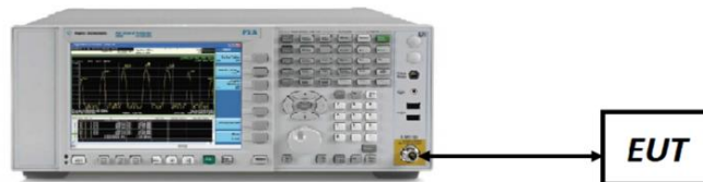
Figure 7-2. Test Instrument & Measurement Setup
