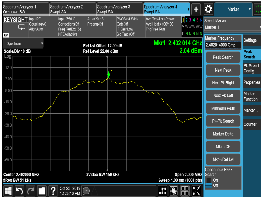
Figure 22 - 2402 MHz, Power Spectral Density
