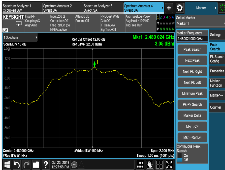
Figure 24 - 2480 MHz, Power Spectral Density
