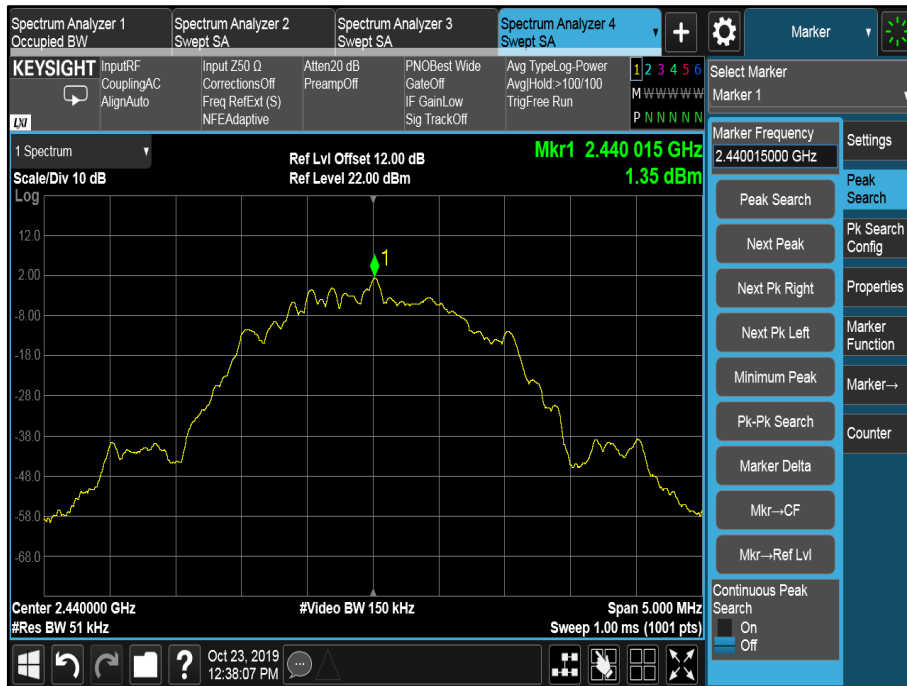
Figure 26 - 2440 MHz, Power Spectral Density
