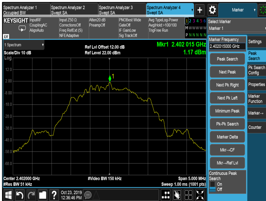
Figure 25 - 2402 MHz, Power Spectral Density
