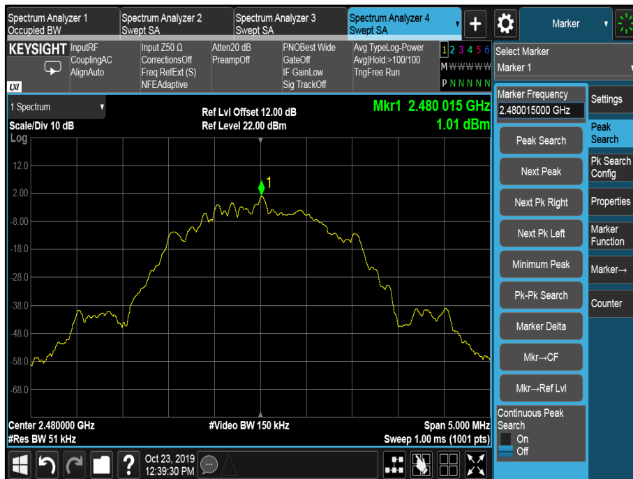
Figure 27 - 2480 MHz, Power Spectral Density
