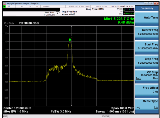
Plot 7-102. PSD Antenna 5b (40MHz BW 11ax Index 8 – RU26 – Ch.46)
