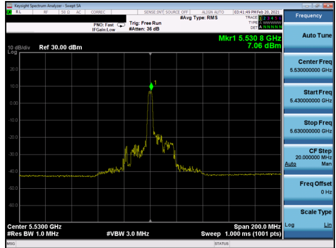
Plot 7-130. PSD Antenna 5b (80MHz BW 11ax Index 18 – RU26 – Ch.106)
