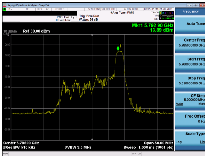
Plot 7-135. PSD Antenna 5b (20MHz BW 11ax Index 8 – RU26 – Ch.157)
