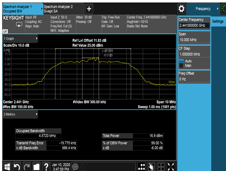
Figure 35 – 2441 MHz – Emission Bandwidth
