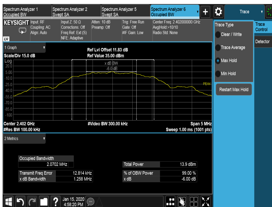
Figure 22 - 2402 MHz – Emission Bandwidth
