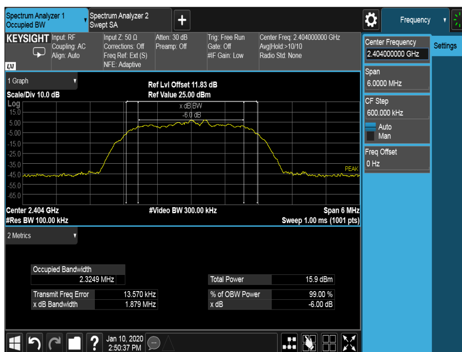
Figure 28 - 2404 MHz – Emission Bandwidth
