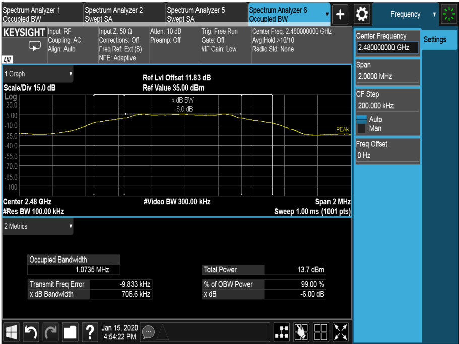
Figure 21 - 2480 MHz – Emission Bandwidth
