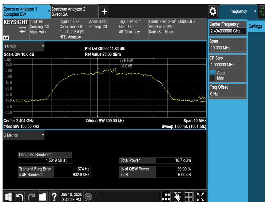
Figure 34 - 2404 MHz – Emission Bandwidth
