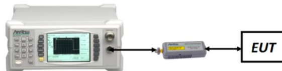
Figure 7-2. Radiated Measurement Setup for Power Meter Measurements
